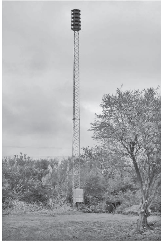
Figure 1.11 A high-directivity voice warning system using an array of toroidal pattern loudspeakers in a civil-defense application. Temperature and wind gradient effects can be noticeable in such applications involving communication outdoors over long distances. (Photo by Mendel Kleiner.)
