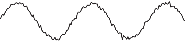
Figure 16.10 Influence of dither on a sine-wave signal when the signal has been D/A-converted and synchronously averaged over a number of periods.
