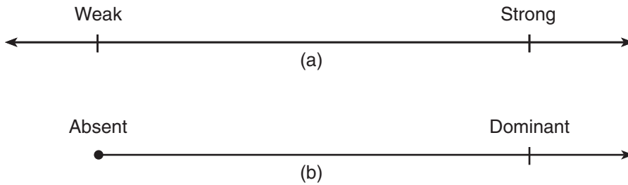
Figure 17.25 Examples of bipolar (a) and unipolar (b) scales for semantic differential tests. The upper scale has open ends, the lower scale has one closed end. Typically two anchors help determine the scale.
