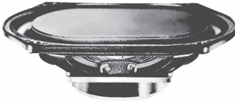
Figure 8.5 Loudspeakers using pyramidal, homogeneous plastic foam diaphragms such as this KEF B139 will tend to have their frequency response affected by quasilongitudinal wave resonances in the diaphragm. (Photo by Mendel Kleiner.)
