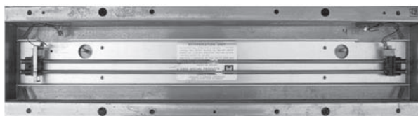
Figure 8.2 Reverberation units such as this one may use the low propagation velocity of longitudinal and torsional waves in metal spring coils to generate the desired delays and reflection patterns needed to synthesize reverberation for guitar amplifier applications. (Photo by Mendel Kleiner.)
