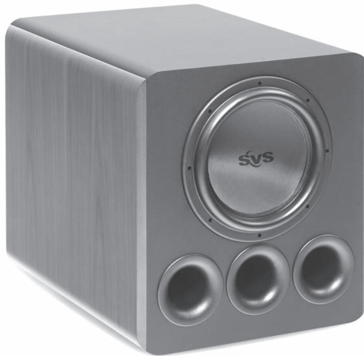
Figure 9.10 Note the flare of the three bass-reflex port openings of this SVSound™ PB12-Plus subwoofer. Many ported loudspeaker enclosures use a flared port to reduce the swooshing noise associated with turbulence generated by turbulence in air at high flow velocities. An application of this technology can be seen in the loudspeaker shown here (photo courtesy of SVSound™ [all rights reserved]).
