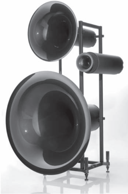
Figure 9.3 Horns are sometimes used to increase the radiation impedance sensed by the loudspeaker diaphragm (photo courtesy of Avantgarde Acoustic GmbH, Germany).
