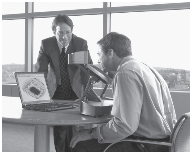
Figure 6.23 The Bose Auditioner® system is a commercial system for auralization using CAD. The binaural room impulse responses are convolved with music or speech so that it is possible to listen to a simulation of what it would be like to listen in the actual room being simulated. Crosstalk cancellation is used to render the binaural signals in this setup (photo courtesy of Bose Corporation).
