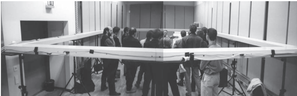
Figure 17.10 An experimental rectangular array for WFS sound reproduction using 256 loudspeakers (photo by Mendel Kleiner).
