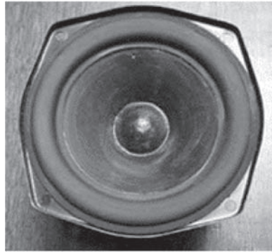
Figure 8.13 Early loudspeakers having a diaphragm made of plastic material, such as this KEF B110, needed to have their diaphragm surfaces treated with viscoelastic compounds to damp the bending wave resonances since the plastics used had small loss factors. (Photo by Mendel Kleiner.)
