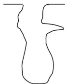
Figure 9.8 Grout distribution in the hole.
