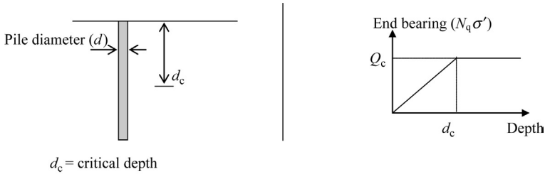
Figure 7.10 Critical depth for end bearing.
