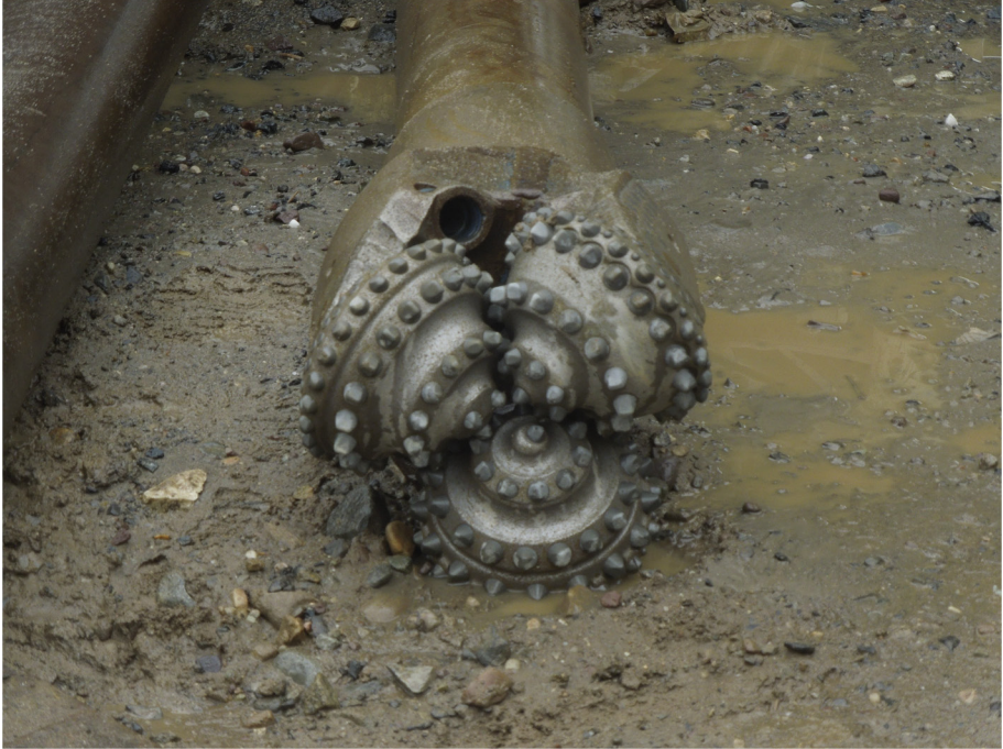
Plate 1.3 Roller bit (Roller bit cut through soil. Water is injected from the hole to keep the roller bit from overheating).
