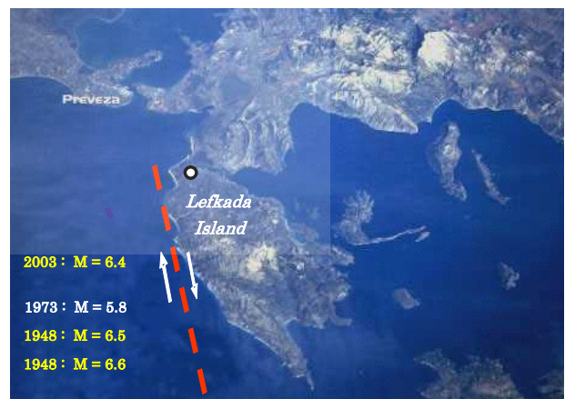
Fig. 1 : Top : The Cefalonia Transform Fault with the fault mechanism of a number of pre-1999 events [2]. Bottom : Satellite view of the Lefkada island and the approximate location of the 2003 rupture of the Transform Fault [1].
