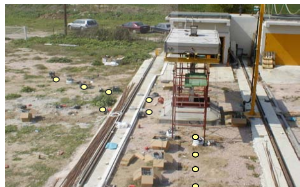
Figure 13. Instrumentation of the surrounding free-field soil.
