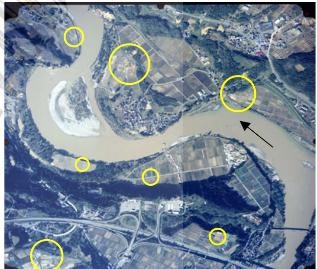
Photo 11: Sand boils on point bars along the Shinano River in Kawaguchi. Circles indicate areas of sand boiling.
