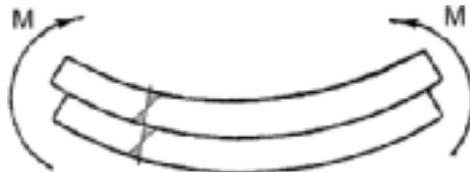
**Fig. 3.5.2.** Beam in Fig. 3.5.1 split along the neutral plane O-O.
