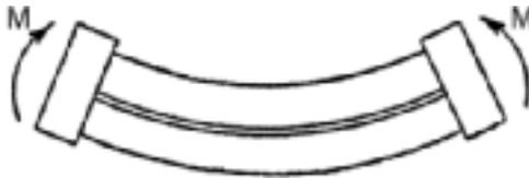
**Fig. 3.5.5.** Split beam with clamped ends.
