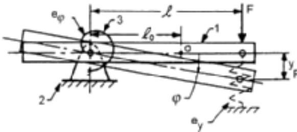
**Fig. 6.3.1.** Reduction of angular compliance to equivalent translational compliance.
