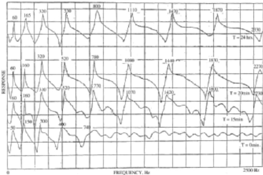
**Fig. 7.4.19.** Response spectra at different times; 10 dB/div, 0 Hz to 2,500 Hz range.
