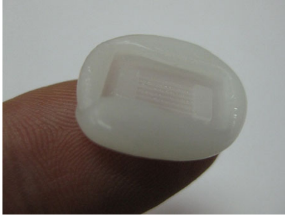
Fig. 12.6 Hot-stamped polycaprolactone substrate, using rapid prototyped part as stamp (see also Fig. 10.16), for obtaining a microfluidic device in final biomaterial for cell growth and motility studies
