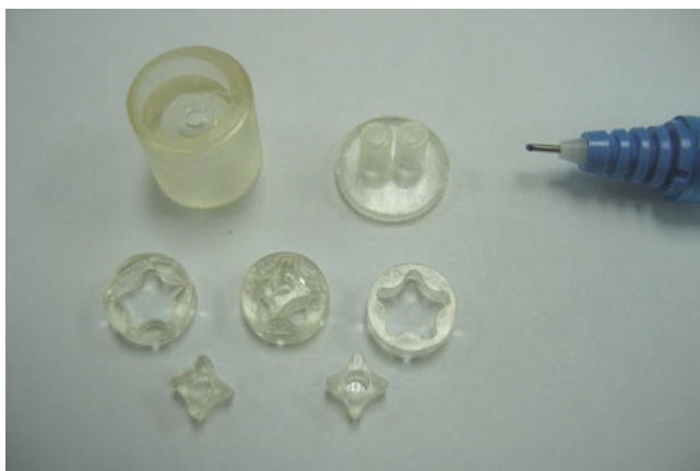
Fig. 10.6 “Gerotor”-type micropump: prototypes of cases and gears for analyzing the tolerances achieved, the assembly process, and the pumping process (Manufactured using laser stereolithography: SLA-3500 Machine 3D Systems)
