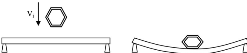
Figure 6.1. Shock of one structure on another structure
