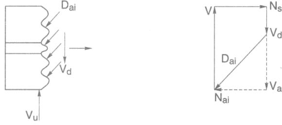
Fig. 3.3-67: Shear transmission in a reinforced crack
