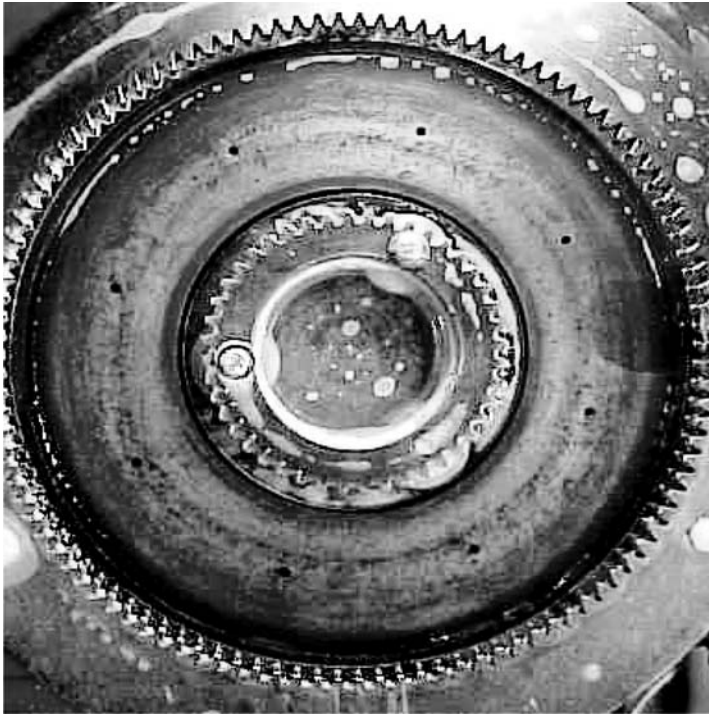
FIGURE 12.12 Radial wear gradient of the diamond wheel.
