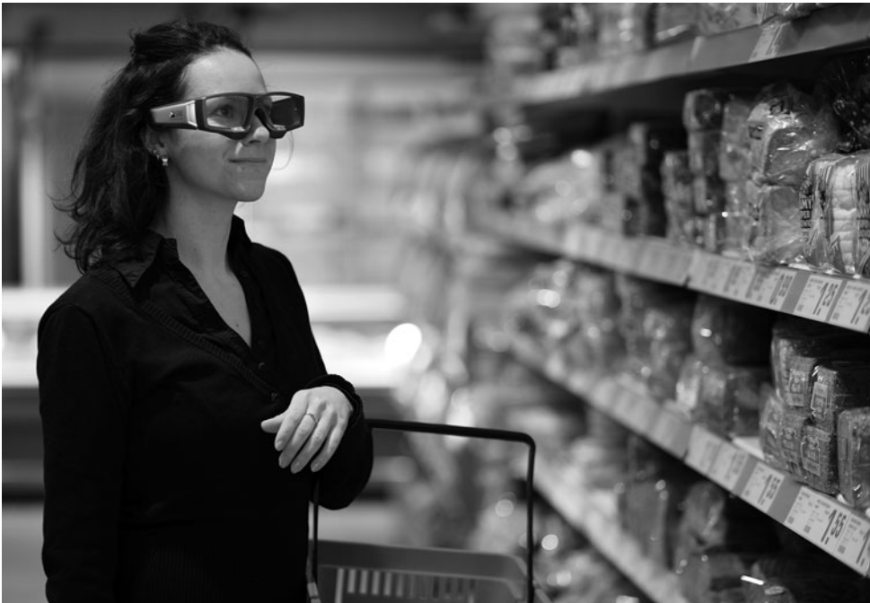
Figure 9.2 SMI's binocular mobile eye-tracking glasses in a shopper research application. 4 Source: http://www.eyetracking-glasses.com/gallery/
