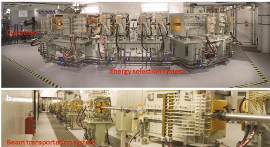
**Fig. 2.1** Cyclotron and energy selection system (a) and a section of the beam transportation system (b) for a proton therapy facility (Courtesy of IBA, SA). Vacuum tube with multiple steering or bending magnets guide and focus the narrow proton beam to treatment rooms
