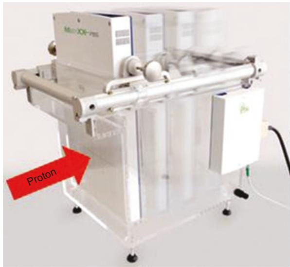
[6]. Lin et al. [26] investigated the feasibility of using a waterproof housing to hold the MatriXX that is scanned in a water phantom (DigiPhant, IBA dosimetry) (Fig. 2.11). This new dosimetry tool could combine point dose, depth dose, and 2D dose distribution in one setup and significantly reduce the time and QA workload. Unfortunately such QA tools are not able to verify the gantry dependent parameters, e.g., current settings of all bending and steering magnets.
