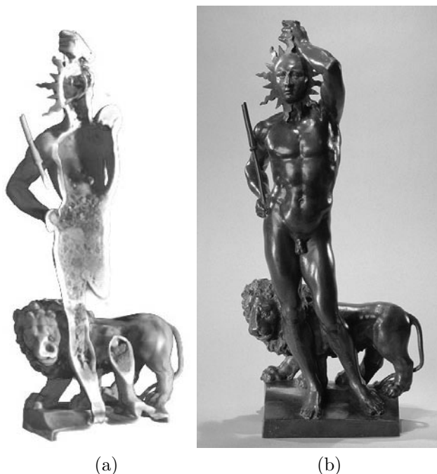
FIG. 13.20. Photo (a) and virtual slice (b) through the bronze sculpture 'Sol (The Sun)' from Rijksmuseum Amsterdam, height 45.7 cm, made by J. van der Schardt (around 1585). The metallic structure, the casting process and repair measures were studied in great detail (Paul Scherrer Institut, 2007).
