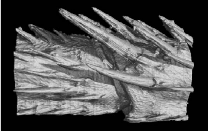
FIG. 6.8. Rendered surface representation of part of a fly's leg obtained in point-projection mode imaging using a laboratory source using the homogeneous-object single-plane retrieval method. The diameter of the leg is \sim 100 \mu\text{m} (Fig. 11 of Mayo et al. 2003, reused with permission).
