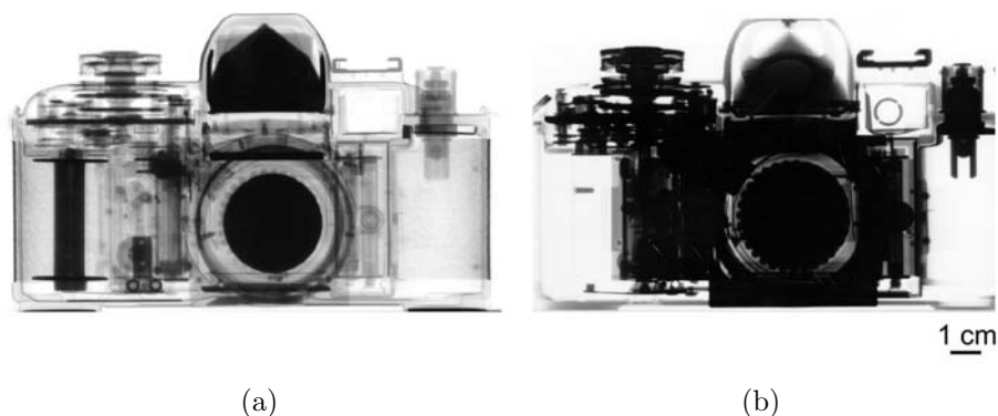
FIG. 13.1. Comparison between radiographic images of a photocamera taken with, (a) thermal neutrons and, (b) X-rays at 150 keV.
