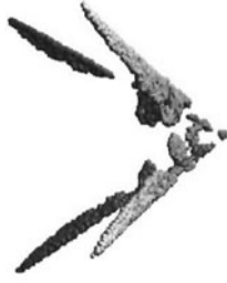
FIG. 6.11. Rendered surface representation of gold balls arranged in a pyramid shape obtained using coherent diffractive imaging at a wavelength of 1.65 nm and sampling the three-dimensional diffraction pattern. The base of the pyramid is 2.5 \mu\text{m} and its height 1.8 \mu\text{m} (Fig. 2b of Chapman et al. 2006, reused with permission).
