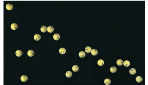
Photo 13.3 The height the tennis ball bounces decreases after each impact because it has a coefficient of restitution less than one and energy is lost with each bounce.
