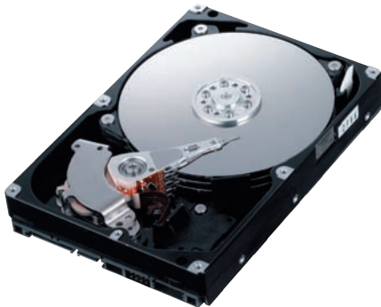
Photo 16.2 The hard disk and pick-up arms of a hard disk computer undergo centroidal rotation.
