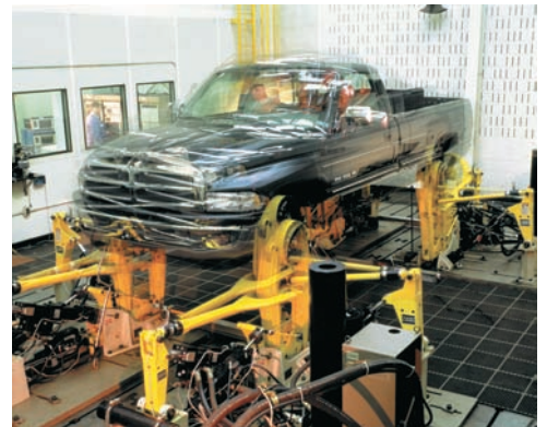
Photo 19.3 This truck is experiencing damped forced vibration in the vehicle dynamics test shown.
