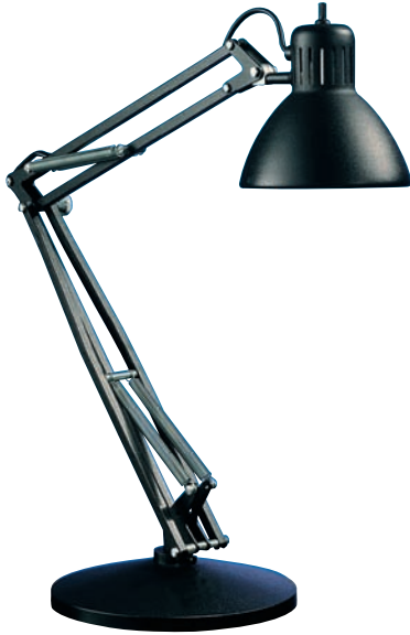
Photo 6.5 The lamp shown can be placed in many positions. By considering various free bodies, the force in the springs and the internal forces at the joints can be determined.
