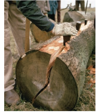
Photo 8.2 Wedges are used as shown to split tree trunks because the normal forces exerted by the wedges on the wood are much larger than the forces required to insert the wedges.
