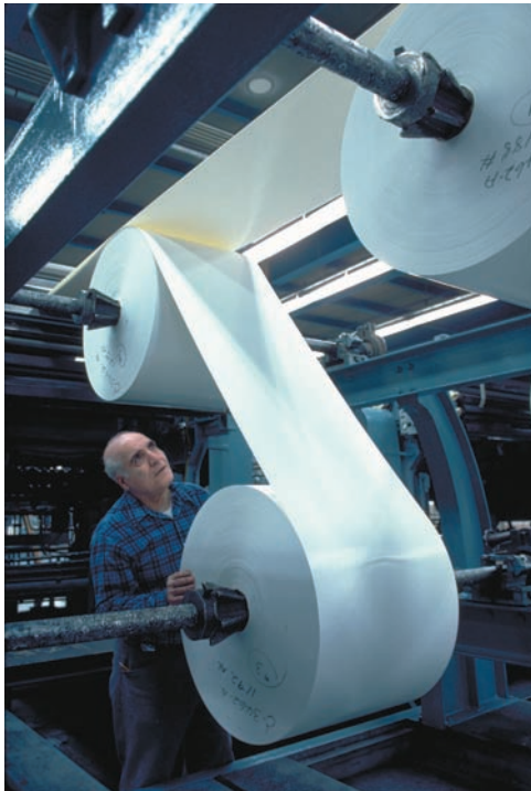
Photo 15.3 If the lower roll has a constant angular velocity, the speed of the paper being wound onto it increases as the radius of the roll increases.
