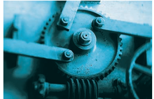
Photo 15.6 The central gear rotates about a fixed axis and is pin-connected to three bars which are in general plane motion.
