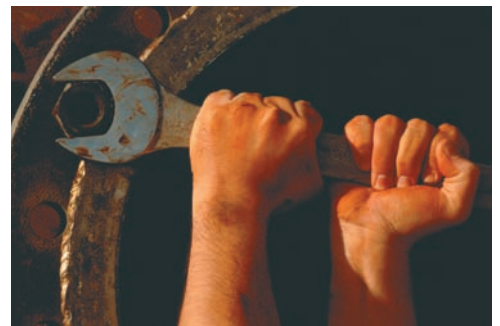
Photo 3.2 The force exerted by each hand on the wrench could be replaced with an equivalent force-couple system acting on the nut.
