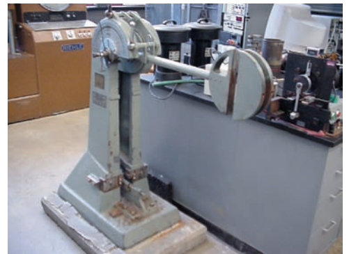
Photo 17.2 A Charpy impact test is used to determine the amount of energy absorbed by a material during impact by subtracting the final gravitational potential energy of the arm from its initial gravitational potential energy.
