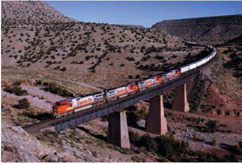
Photo 11.5 The passengers in a train traveling around a curve will experience a normal acceleration towards the center of curvature of the path.
