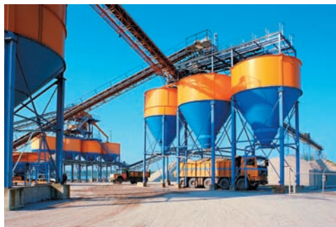
Photo 5.2 The storage tanks shown are all bodies of revolution. Thus, their surface areas and volumes can be determined using the theorems of Pappus-Guldinus.
