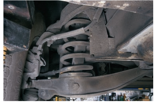
Photo 19.2 The automobile suspension shown consists essentially of a spring and a shock absorber, which will cause the body of the car to undergo damped forced vibrations when the car is driven over an uneven road.
