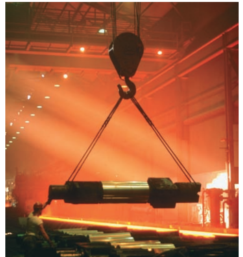
Photo 2.1 As illustrated in the above example, it is possible to determine the tensions in the cables supporting the shaft shown by treating the hook as a particle and then applying the equations of equilibrium to the forces acting on the hook.
