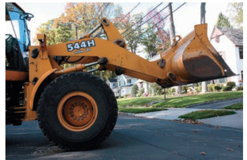
Photo 4.2 In Chap. 6, we will discuss how to determine the internal forces in structures made of several connected pieces, such as the forces in the members that support the bucket of the tractor of Photo 4.1.
