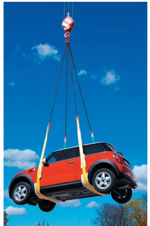
Photo 2.2 While the tension in the four cables supporting the car cannot be found using the three equations of (2.34), a relation between the tensions can be obtained by considering the equilibrium of the hook.
