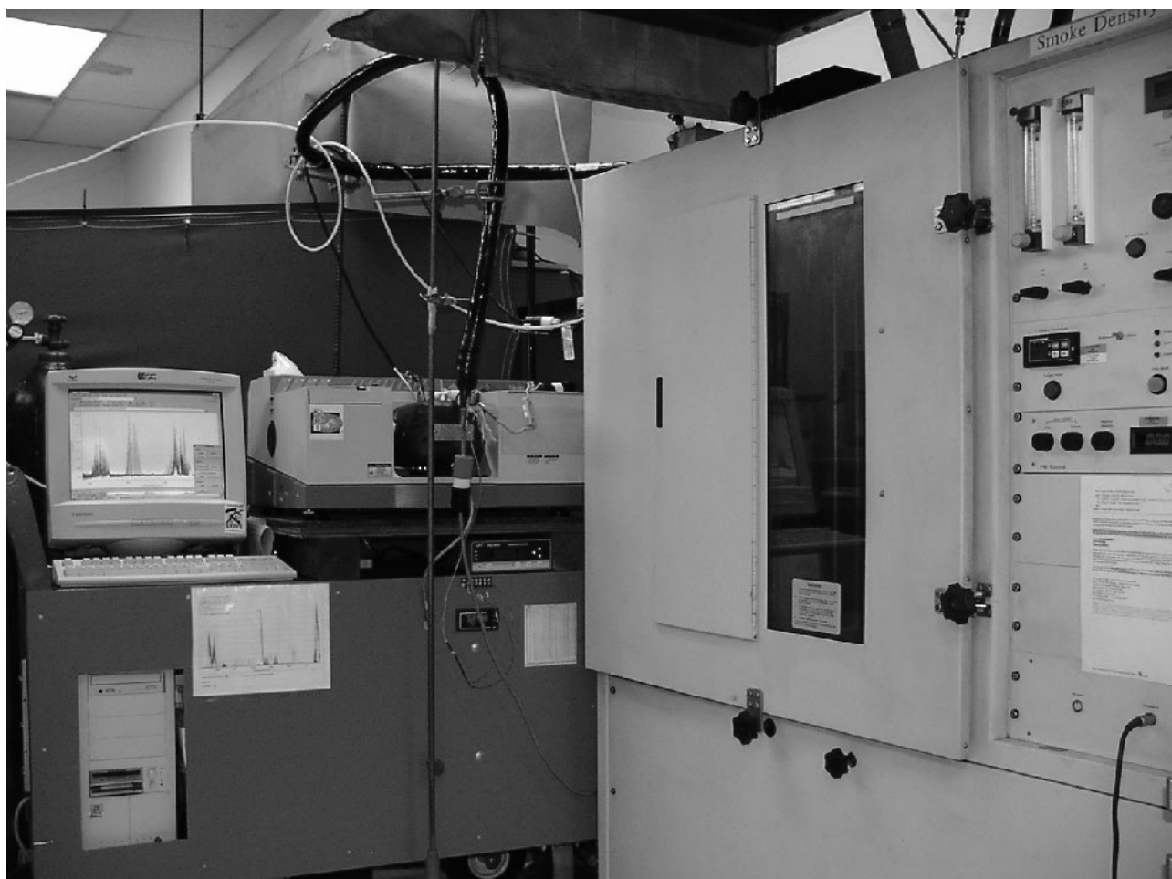
FIGURE 10.7 NBS smoke chamber with FTIR spectrometer for gas analysis.
