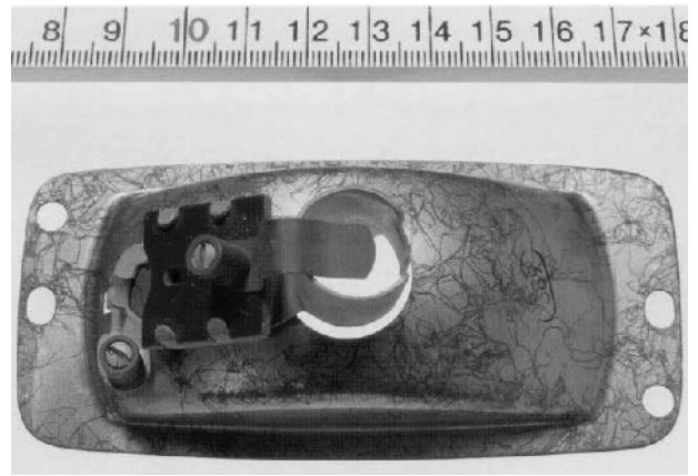
FIGURE 18.5 Filiform corrosion on varnished steel subject to moist indoor atmospheres. [Source: E. D. D. During, Corrosion Atlas , 3 rd Ed. New York: Elsevier, p. 285, 1997]
