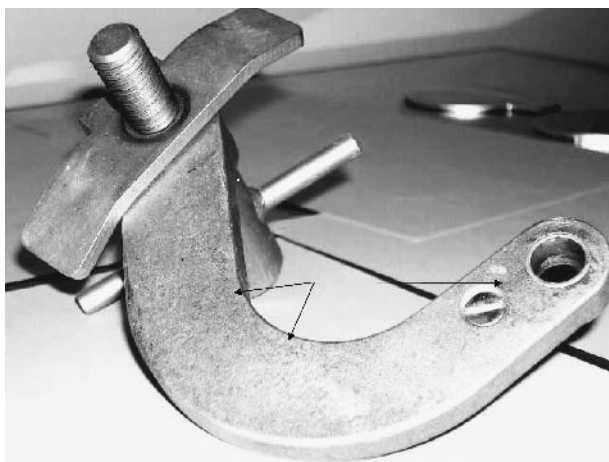
FIGURE 27.4 The surface of this stainless steel part was cleaned with steel wool. The resulting contaminated surface rusted while the part was in use.
