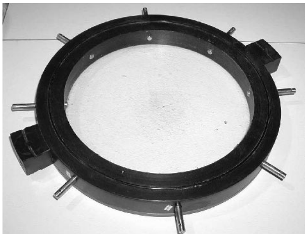
FIGURE 11.8 A photograph of a Wenner eight-pin electrical resistivity measurement cell.
