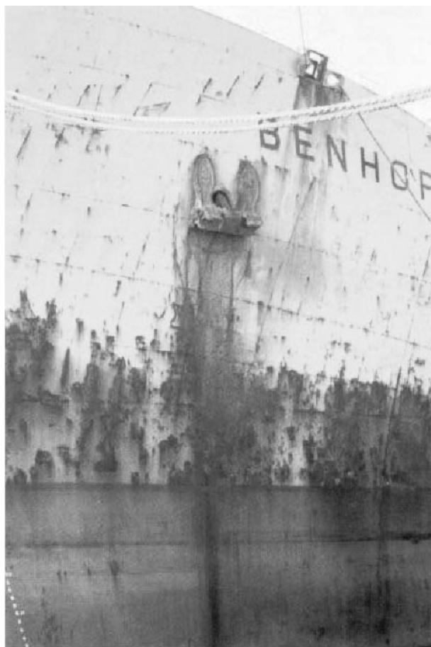
FIGURE 18.2 Alkyd coating (2–3 coats) on steel exposed to a marine environment. Increased corrosion damage near the water line illustrates the unsuitability of alkyd coatings for immersion service. [Source: E. D. D. During, Corrosion Atlas , 3 rd Ed. New York: Elsevier, p. 293, 1997]
