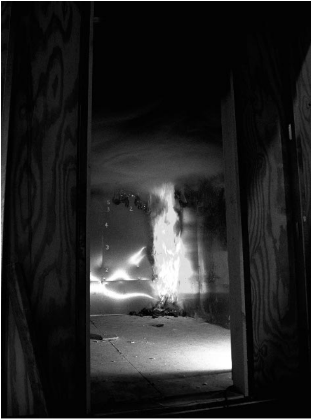
FIGURE 10.6 ISO 9705 room/corner test in progress.
