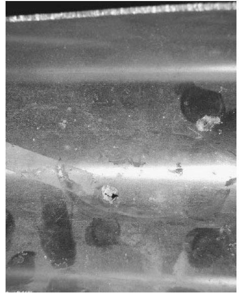
FIGURE 27.8 The deposits baked on by hot spots on the pipe surface created corrosion and perforation under the deposits. This photograph is an enlargement for one of the deposits seen in Figure 27.7.
