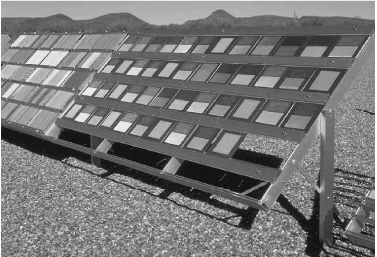
FIGURE 19.6 Paint test panels exposed at 45 degrees facing south in Arizona. [Picture courtesy of Atlas Weathering Services Group]
