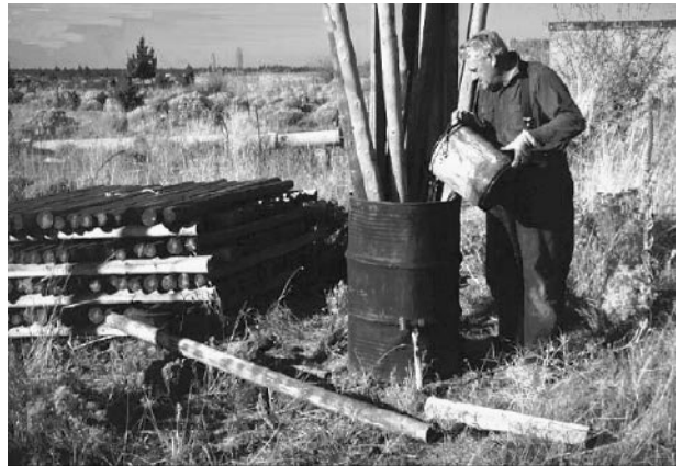
FIGURE 15.8 Brushing and soaking of wood in preservatives produce a relatively shallow zone of protection.
