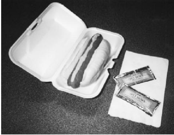
FIGURE 26.30 The Heinz condiment pouches. A 2-mil structure of: lacquer/print/Mylar ® MC2 PET/adhesive/LDPE [26]. The Mylar ® MC2 PET layer consists of a laminate of PVDC/Clear PET/Aluminum/PVDC. [Source: With permission of Dupont.]
