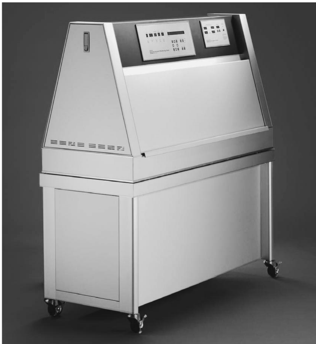
FIGURE 19.16 Typical fluorescent lamp weathering chamber. (Picture Courtesy of Q-Panel Company)
