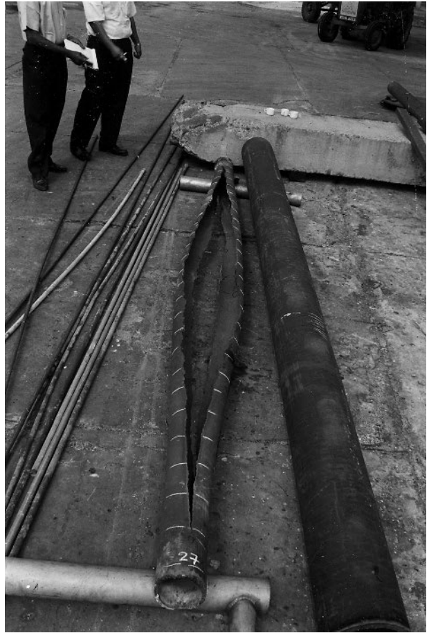
FIGURE 2.10 The length containing the cracks cut from the reformer tube.
