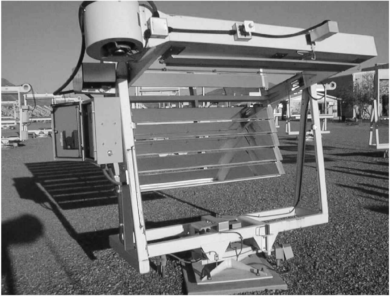
FIGURE 19.10 Solar Fresnel mirror exposure apparatus in Arizona. [Picture courtesy of Atlas Weathering Services Group]
