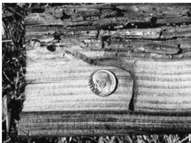
FIGURE 15.6 Adult beetles, such as this golden buprestid beetle ( Buprestis aurulenta ), leave small exit holes on the wood surface, but can cause substantial internal damage.
