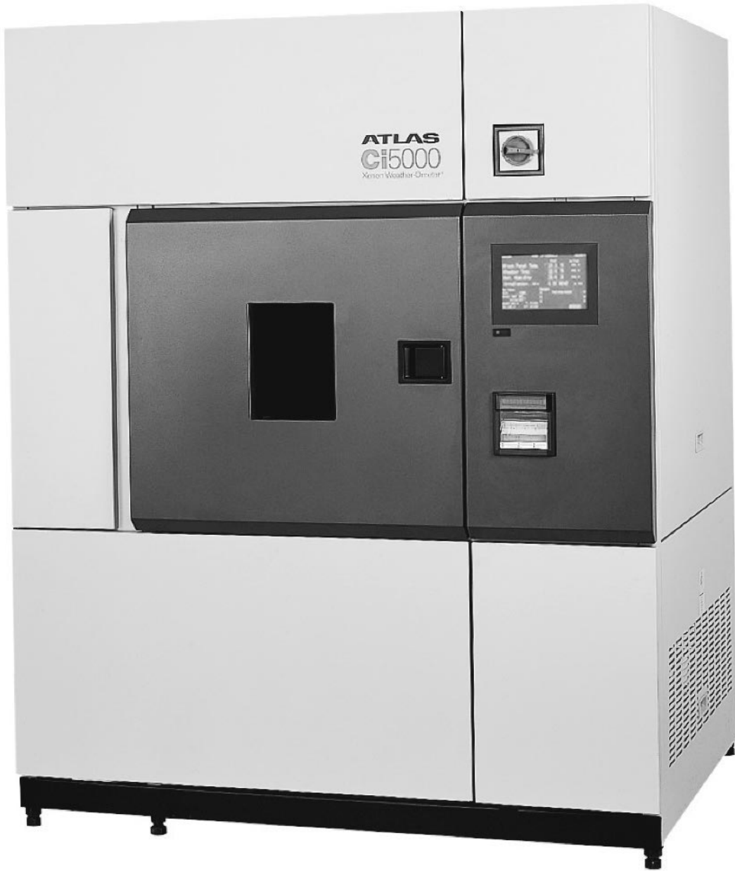
FIGURE 19.15 Typical xenon arc type weathering chamber. (Picture courtesy of Atlas Materials Testing Technology LLC)
