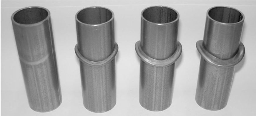
Fig. 6 Typical modes of deformation that may develop during asymmetric compression beading of thin-walled commercial S460MC tubes with different slenderness ratios
