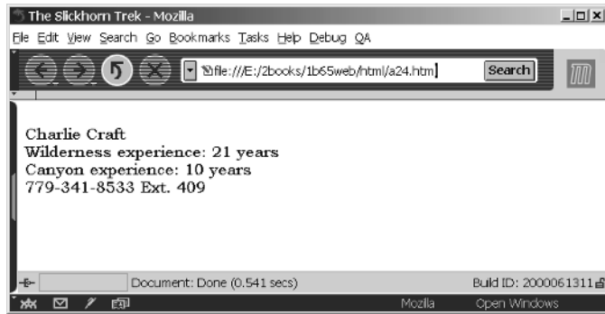
Figure A4.1 Use <br> for line breaks not followed by a blank line.
