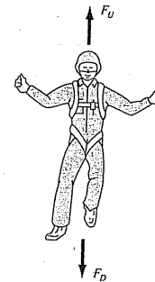
FIGURE 1.2 Schematic diagram of the forces acting on a falling parachutist. F_D is the downward force due to gravity. F_U is the upward force due to air resistance.
