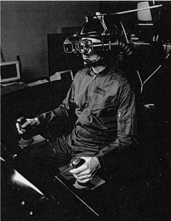
FIGURE 3.2. Helmet-mounted display system (courtesy of CAE Electronics Ltd., St.-Laurent, Quebec, Canada.)
