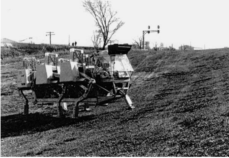
FIGURE 1.10. The OSU ASV. An example of a six-legged walking machine (courtesy of Prof. K. Waldron. Reproduced with permission of The MIT Press.)
