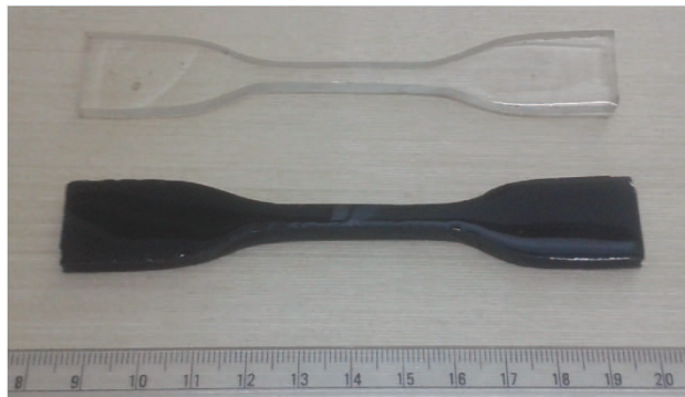
Fig. 23.1: Macro-photographs of neat (E-0-CNT) and filled (E-1CNT) epoxy
