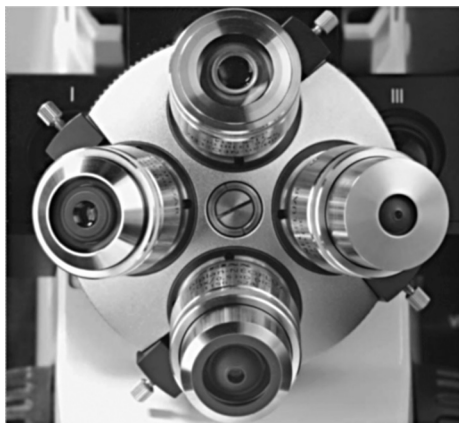
FIGURE 3.8 Parfocal arrangement of four different objectives on a revolving turret. Once any of the four objectives is properly focused on the specimen, one need not adjust the focus when any other objective is brought into position. (Photo courtesy of Carl Zeiss Microimaging, LLC. With permission.)
