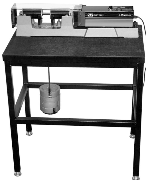
FIGURE 11.4 Photograph of the R. R. Moore rotating-beam fatigue-testing system. The specimen can be rotated up to 9999 complete stress cycles per minute with bending stress applied by means of dead weights. (Photo courtesy of Instron Corporation. With permission.)
