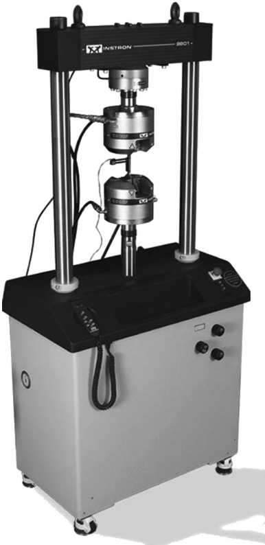
FIGURE 11.5 100 kN servohydraulic machine for high-cycle fatigue testing of metallic and composite materials used in airplane fuselages. (Photo courtesy of Instron Corporation. With permission.)
