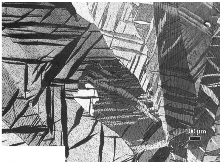
FIGURE 3.20 Photomicrograph of pure metal zinc. The grains are elongated in this specimen. The presence of mechanical twins inside the grains may additionally be noted. (Photo courtesy of ASM International, Materials Park, OH. With permission.)
