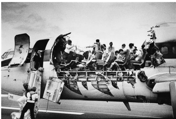
FIGURE 11.11 Photograph of the fuselage of the Aloha Airlines Boeing 737 aircraft after its roof was torn off. The accident was caused by metal fatigue (repeated compression and decompression cycles, numbering 89,680) and crevice corrosion (the plane was primarily operating in saltwater-saturated climate).
