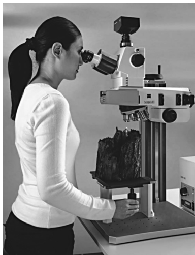
FIGURE 3.7 An optical microscope with a stage to accommodate very large specimens. (Photo courtesy of Carl Zeiss Microimaging, LLC. With permission.)
