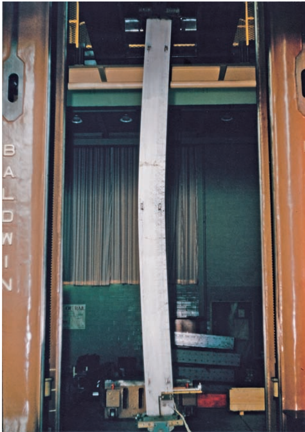
Photo 16.1 Test column that has buckled
