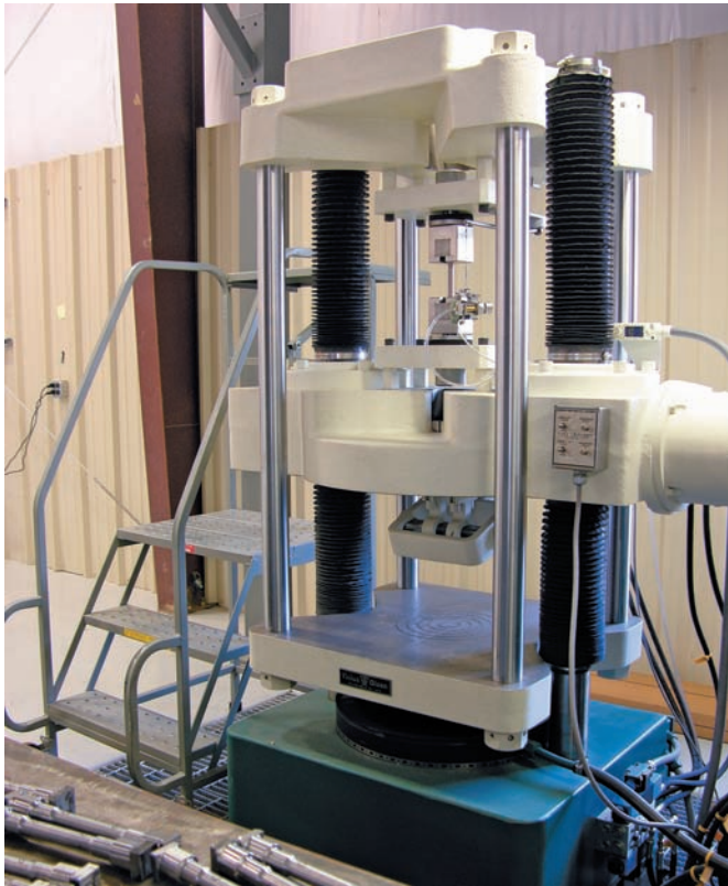
Photo 9.2 This machine is used to test tensile-test specimens, such as those shown in this chapter.
