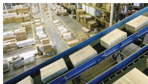
Photo 4.8 The coefficient of static friction between a package and the inclined conveyor belt must be sufficiently large to enable the package to be transported without slipping.
