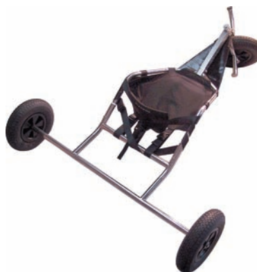
Photo 11.1 For the sport buggy shown, the center portion of the rear axle is in pure bending.
