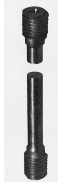
Photo 9.5 Tested specimen of a brittle material.
