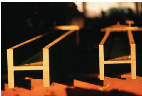
Photo 7.1 Appendix B tabulates data for a small sample of the rolled-steel shapes that are readily available. Shown above are two examples of wide-flange shapes that are commonly used in the construction of buildings.
