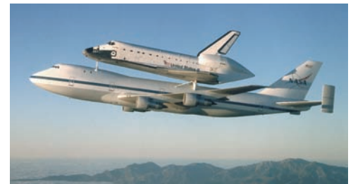
Photo 5.4 To predict the flight characteristics of the modified Boeing 747 when used to transport a space shuttle, the center of gravity of each craft had to be determined.
