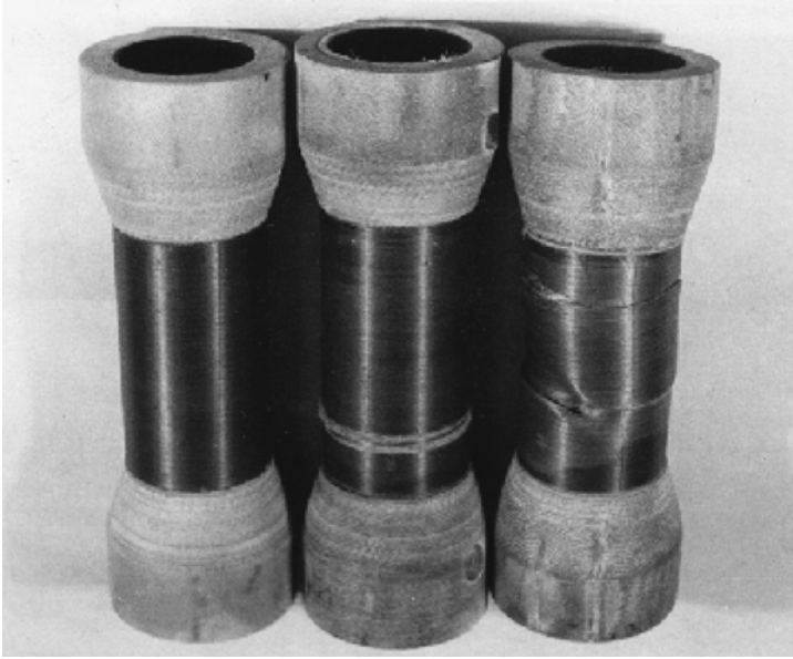
Fig. 6.4. Carbon-epoxy test tubular specimens made by circumferential winding (the central cylinder failed under axial compression and the right one under torsion).
