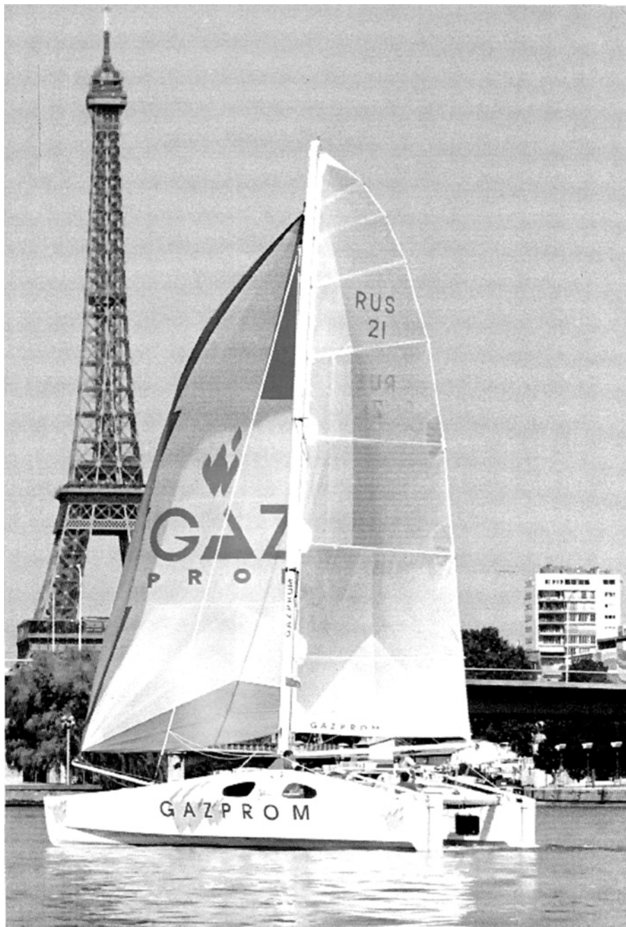
Fig. 1.18. Catamaran yacht Ivan-30 made from carbon-epoxy composite by hand lay-up. Courtesy of CRISM.
