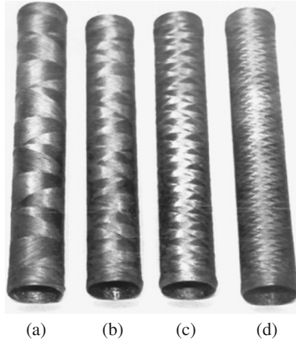
Fig. 5.26. Filament-wound cylinders with various numbers n_T of T -segments: n_T = 2 (a), 4 (b), 8 (c), and 16 (d).
