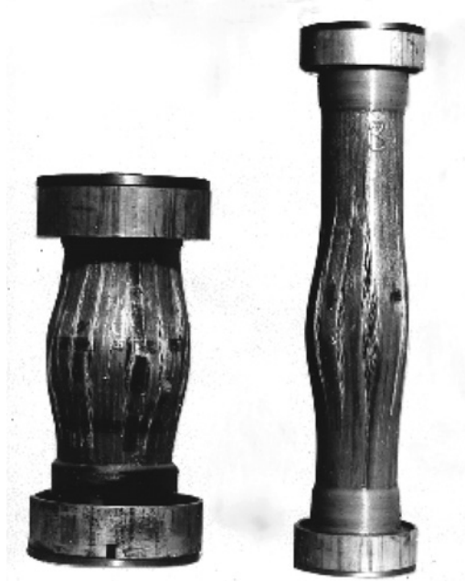
Fig. 6.12. Failure modes of a unidirectional glass-epoxy composite under longitudinal compression.
