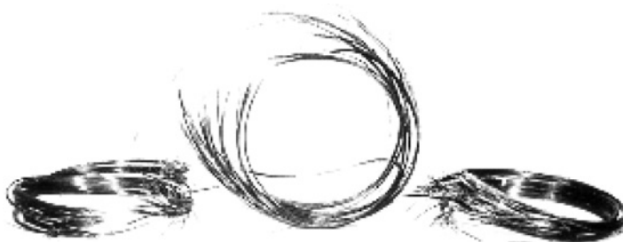
Fig. 3.48. Failure modes of unidirectional rings.
