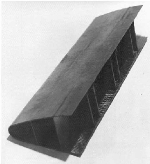
Fig. 4.82. A composite leading edge of an aeroplane wing made of carbon fabric by lay-up method. Courtesy of CRISM.
