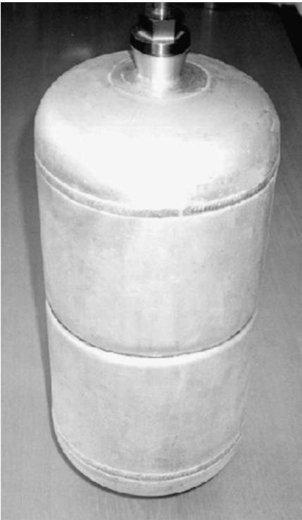
Fig. 4.3. Aluminum liner for a composite pressure vessel.
