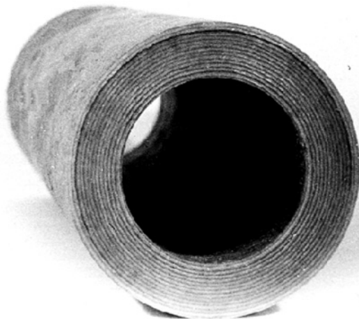
Fig. 4.1. Laminated structure of a composite pipe.
