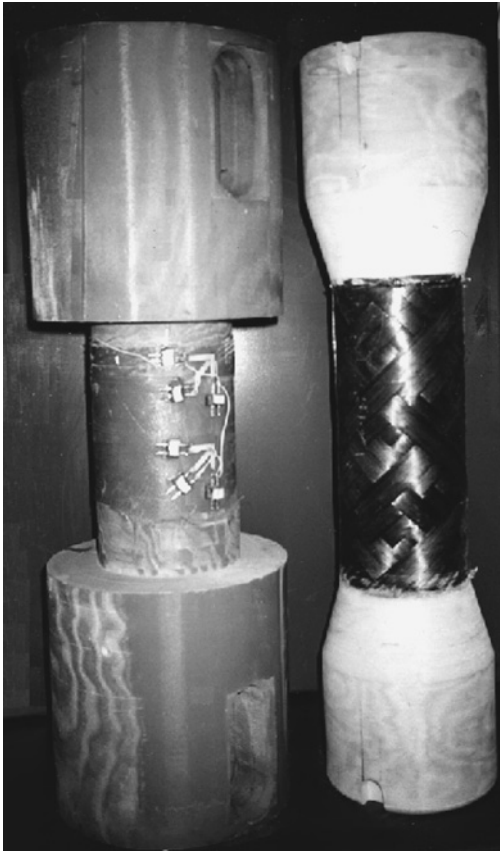
Fig. 6.19. Segments of composite drive shafts with test fixtures. Courtesy of CRISM.
