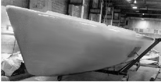
Fig. 4.81. A composite body of a boat made of fiberglass fabric by lay-up method. Courtesy of CRISM.
