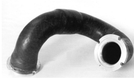
Fig. 4.67. A curved angle-ply pipe made by deformation of a filament-wound cylinder.
