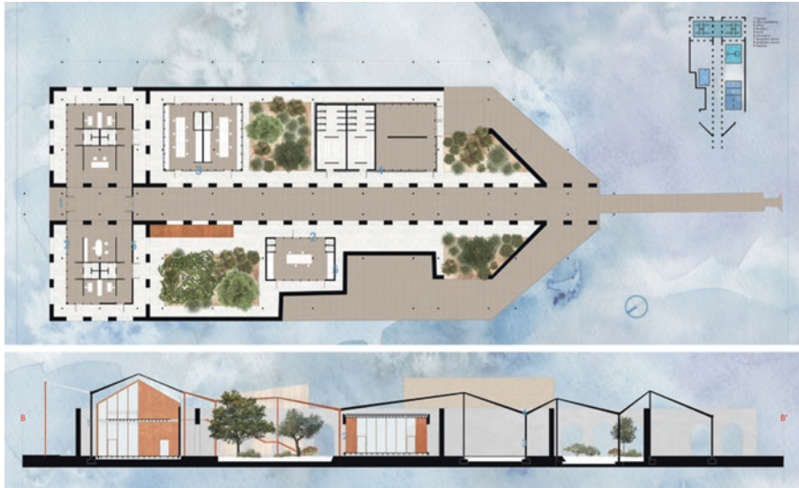
Figs. 8.32 and 8.33 Project plan with main axis to the sea, courtyards, and workshop. The spaces of research present a double ventilated and massive skin
