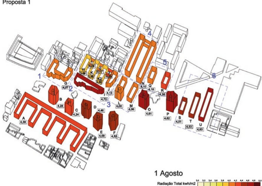
Fig. 6.30 Overall analysis of proposal 1 for the typical day of the cooling station
