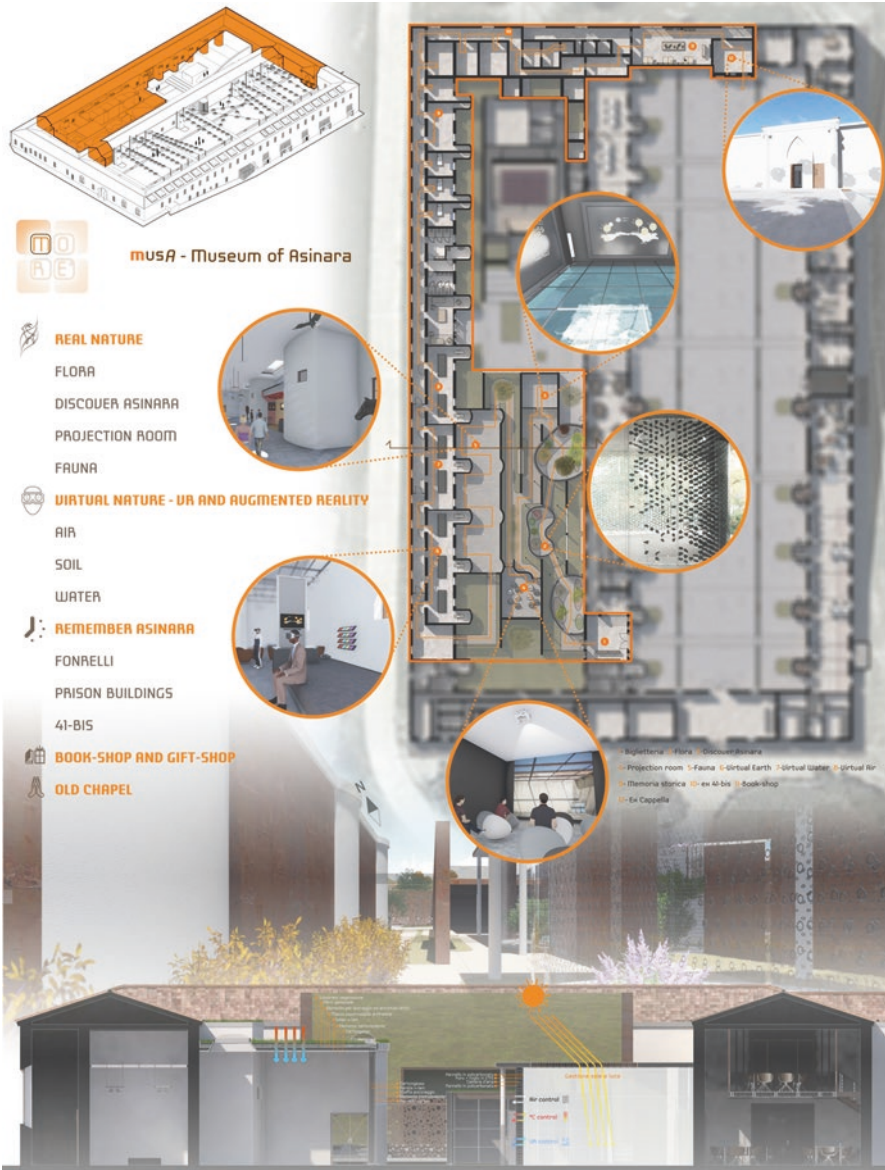
Fig. 8.28 Summary of concept design of Fornelli Cultural Hub: the activities distribution, the exposition roadmap. Bioclimatic strategies to optimize environmental comfort design, improving quality of daylighting, and integrating natural resource (green and water) and renewables
