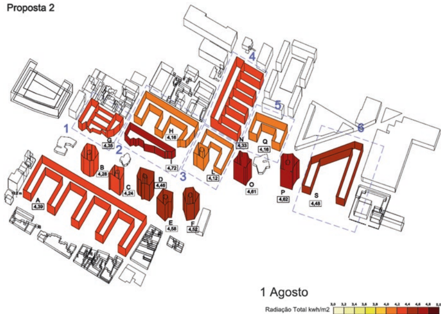
Fig. 6.31 Overall analysis of proposal 2 for the typical day of the cooling season
