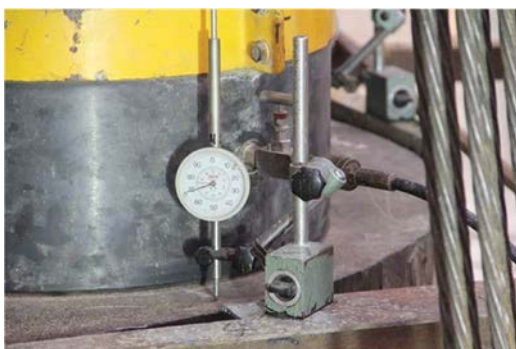
Figure 13.14 Dial gauge measurement of pile head settlement.
