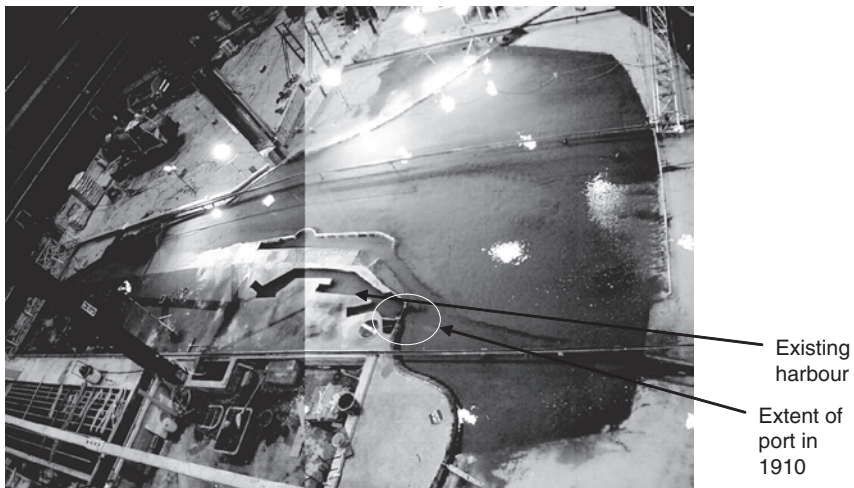
Figure 11.19 A panoramic view of the physical model with the existing and the future (now built) Le Havre harbour (courtesy of Sogreah, Grenoble)
