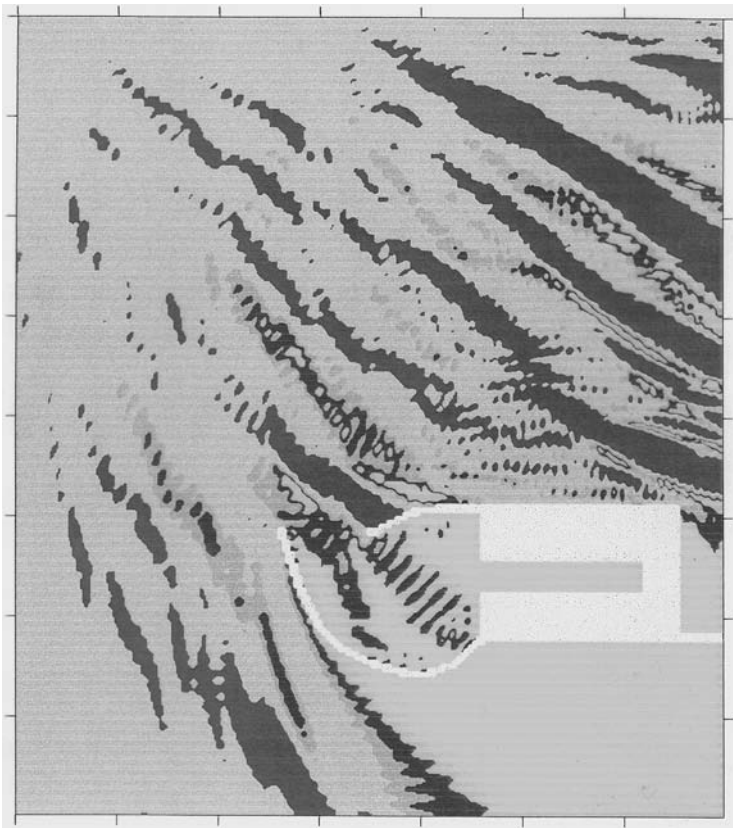
Figure 12.20 Computed wave heights in Option E demonstrating much better wave-energy absorption for the berthing area. The orientation and shading are the same as in Figure 12.19 (courtesy of Halcrow)
