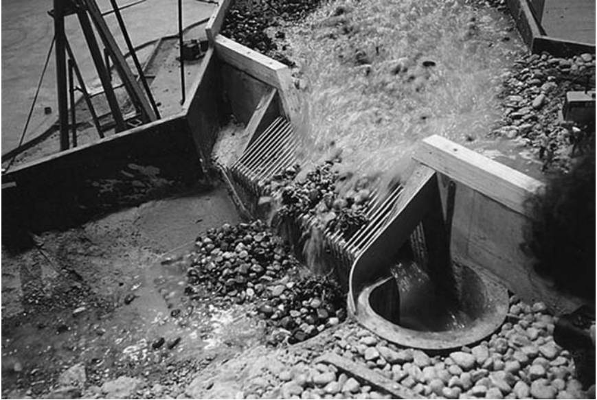
Figure 8.8 The diversion intake in the Arve model, M_I = 27 (courtesy of Sogreah, Grenoble)
