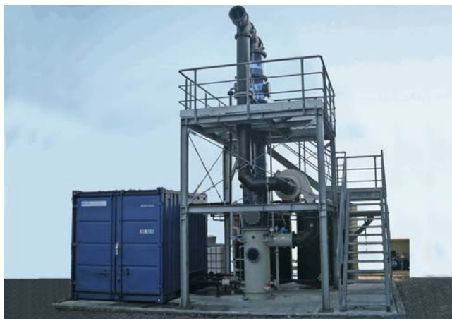
Figure 6-4. Picture of ENVIMAC test plant, shown as drawing in Fig. 6-3, for investigation of packings under normal conditions. d_S = 0.6 m, H = 3.2 m, system: air/water
