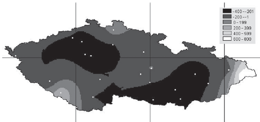
Fig. 10.4 Spatial distribution of annual 30-year average R-ET(Reed) in millimetres for the Czech Republic
