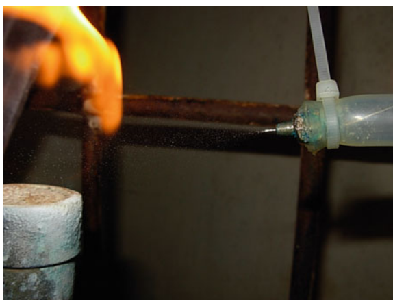
Fig. 4.2 Example of an atomization device developed in laboratory to produce a spray, which is driven to the pilot flame
