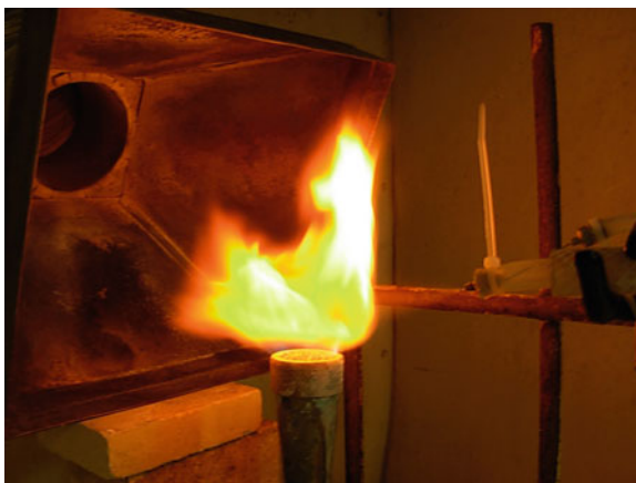
Fig. 4.6 Scheme of the main flame created after the contact of the atomized precursor solution with the pilot flame (Bunsen burner)
