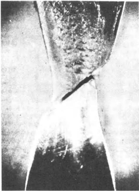
Figure 3: Macroscopic shearing in \theta strengthened crystals. After necking (and load maximum) macroscopic localized shear sets in at nearly 45 degrees to tensile axis on the material plane of maximum shear (After Chang and Asaro [2]).
