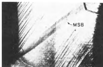
Figure 2: Coarse slip bands (CSB) and macroscopic shear bands (MSB) in a \theta' strengthened crystal tested at 298 K (After Chang and Asaro [2]).
