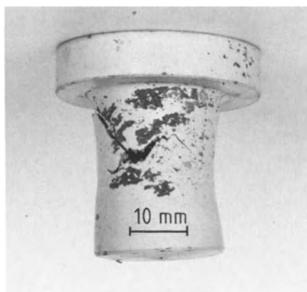
Fig. 17. TiAl-specimen, deformed at 990 °C by small-cup drawing test
