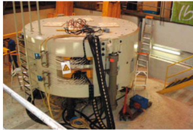
Fig. 17.12 Cyclotron Arronax installed at the Regional Center for Research in Cancerology in Nantes (France). This cyclotron accelerates protons, deuterons ( ^2\text{H} nuclei) and alpha particles (He nuclei) up to an energy of 70 MeV in order to produce radioisotopes for nuclear medicine [Source: Ion Beam Application]
