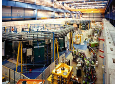
Fig. 17.11 The two cyclotrons CSS1 and CSS2 of GANIL (Grand Accélérateur National d'Ions Lourds, Caen, France). Of a radius of 3 m each, they are connected in series. The intensity of the magnetic field is 0.4 to 0.95 T and the electric-field frequency is 7–14 MHz. The maximum kinetic energy at the output of CSS2 is 95 MeV par nucleon [Source: CNRS/IN2P3]
