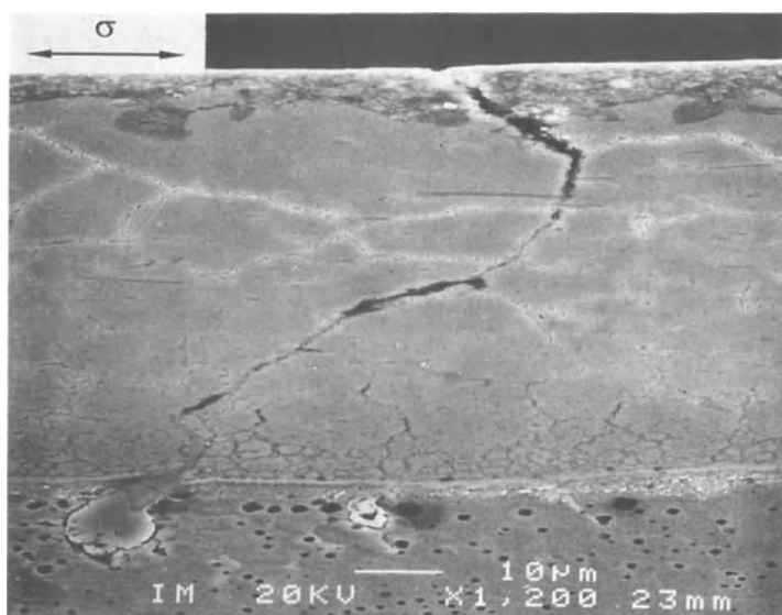
Figure 4. Intergranular crack in the austenitic layer propagating into the ferritic core in semi-coated specimen C2 tested in TMF-IP with \Delta\epsilon_t=1.44\% between 300 and 600°C.
