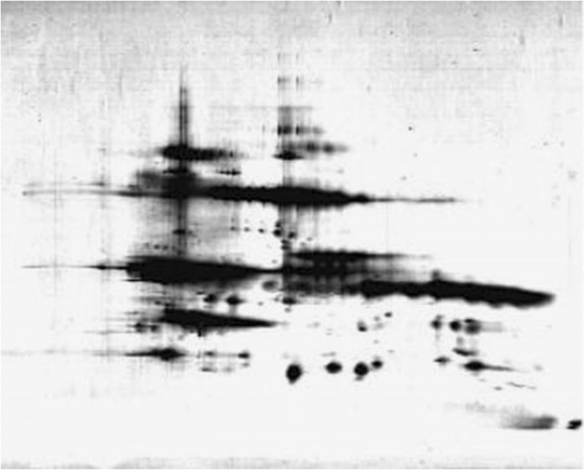
Fig. 4.7. Electrophoretogram of goat's milk in two-dimensional electrophoresis (pH 4–8 from left to right, molecular weight 220 kDa to 10 kDa from top to bottom). Protein spots have been identified by matrix-assisted laser desorption/ionization–time-of-flight mass spectrometry.
