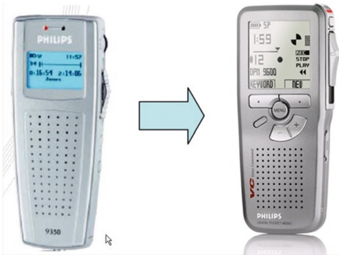
Fig. 3.7 Previous and environmentally redesigned Digital Pocket Memo
