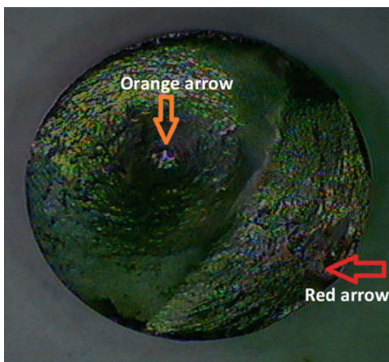
Fig. 14 Fracture surface of a cold processed spring, as seen in a stereo microscope
