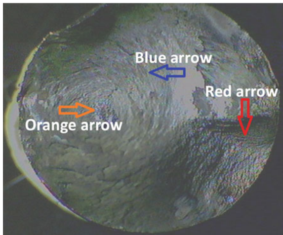
Fig. 9 Fracture surface of hot processed spring, as seen in a stereo microscope
