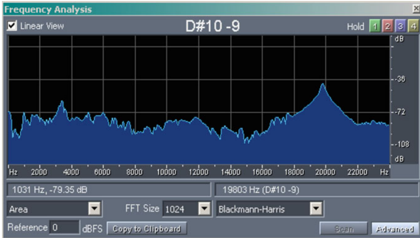
Fig. 7 Measurement's system response to the pulse extinction
