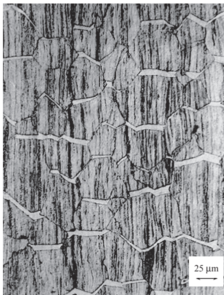
Figure 52 Denuded zones formed perpendicular to the tensile direction in a hydrated Mg-0.5 wt% Zr alloy at 400 °C and 2.1 MPa [262].
