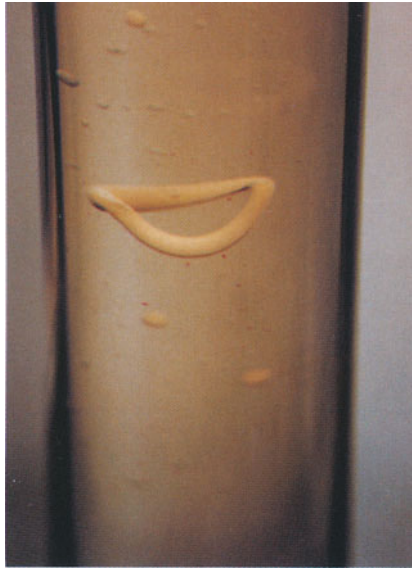
Plate IX.8.4. [Baumann, Joseph, Mohr and Renardy, 1992, American Institute of Physics] Vortex ring of 1000 cS silicone oil with trace amounts of surfactant (Igepal) falling in soy bean oil after blow-out.
