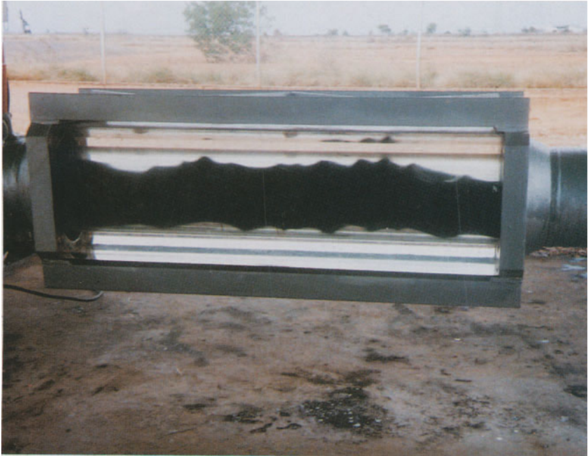
Plate V.2.3. Core-annular flow of oil lubricated by water in a pipe of diameter 8" and test loop of length 1km at San Tome, Venezuela. The water fraction is approximately 10%. The oil is Zuata. At 30°C, the viscosity is 80,000 mPa.s. This photograph was supplied by INTEVEP, SA.
