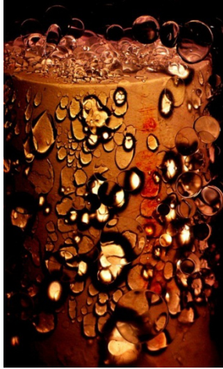
Figure 18.1. Photograph illustrating imbibition in a rock core. The bubbles are the displaced non-wetting phase. Picture from drahellkat.deviantart.com.
