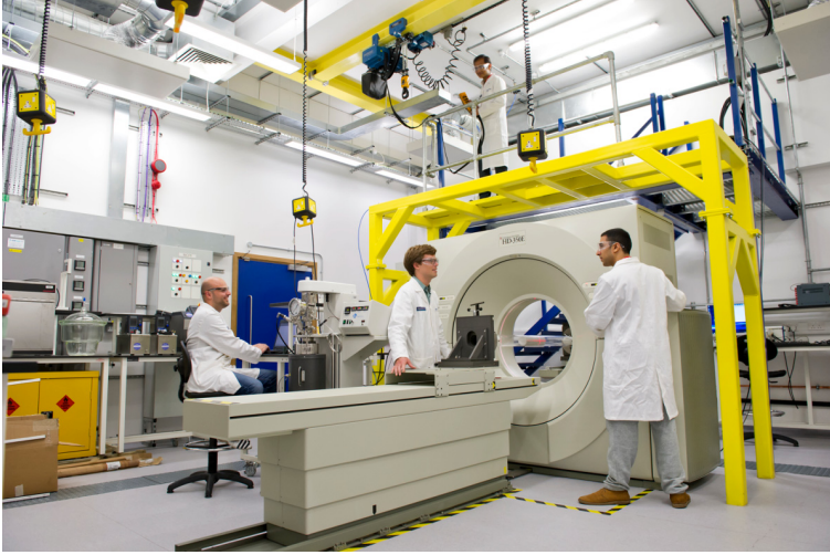
Figure 14.2. A photograph of the apparatus at Imperial College used to measure relative permeability.
