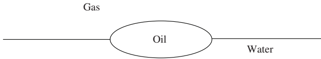
Figure 15.2. The equilibrium arrangement of a small droplet of oil floating on water in the presence of a gas. Here the spreading coefficient is negative and no oil film forms between the gas and water.
