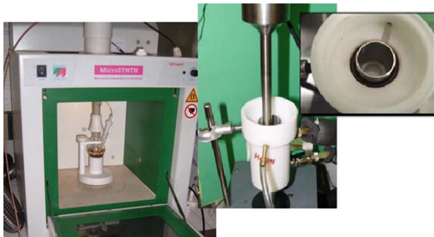
Fig. 2.5 Apparatus for simultaneous US/MW irradiation and detail of immersion horn (25 kHz) inserted in the cavitating tube (19 kHz); the inset shows the latter as seen from the top (Reprinted from Cravotto et al. (2008) with permission from Elsevier)
