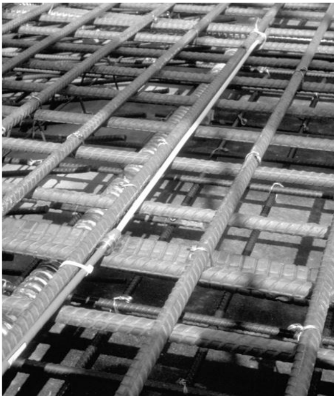
Figure 3-7. SOFO sensor installed on a rebar. The plastic pipe contains the coupled measurement fiber and a free un-coupled reference fiber. Metallic anchors at both ends of the white plastic pipe define the gauge length (Source: Daniele Inaudi, reproduced with permission).
