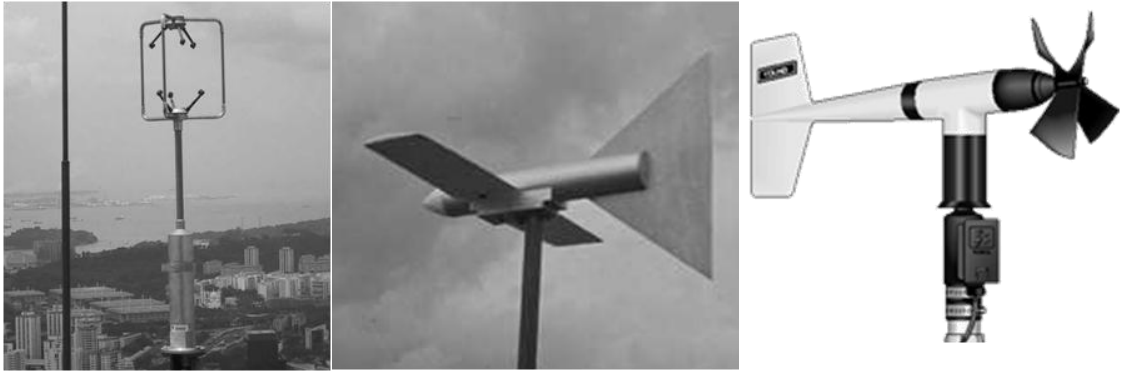
Figure 3-6. Anemometer types: sonic, pitot tube/vane, ‘windmill’
