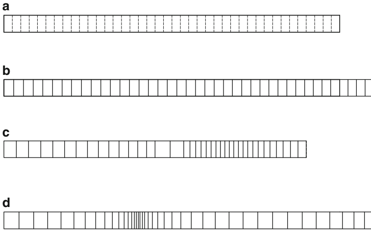
Fig. 8.7 Natural modes of a bar under axial vibration: (a) undeformed configuration; (b) first mode; (c) second mode; (d) third mode
