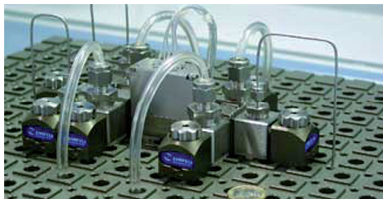
Fig. 4.2. Modular microstructure system (courtesy of of EHRFELD MICROTECHNIK BTS).
