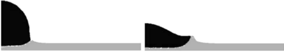
Fig. 10.10. Impact of a droplet on a thin layer at yet lower \text{Re} = 40 . Dimensionless times are t = 0.5 and t = 1.5 . Resolution as in Fig. 10.9. Reprinted with permission from Josserand and Zaleski (2003). Copyright 2003, American Institute of Physics.
