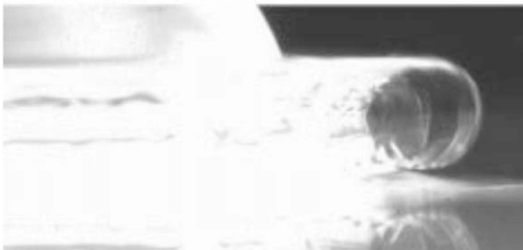
Fig. 10.12. Detail of a spiralling corolla after impact of a glycerine droplet ( Re \sim 1900 , We \sim 2200 , \rho/\rho_a \sim 840 , \mu/\mu_a = 940 ) at dimensionless time t = 0.343 . Reprinted with permission from Thoroddsen (2002).
