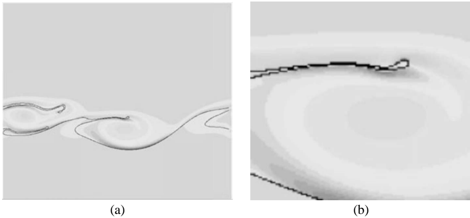
Fig. 9.12. (a) Typical high-resolution simulation. The colors indicate the vorticity. (b) Detail of simulation showing the end rim and a “Kelvin–Helmholtz roller” trapped below the sheet. See plate section for color version.
