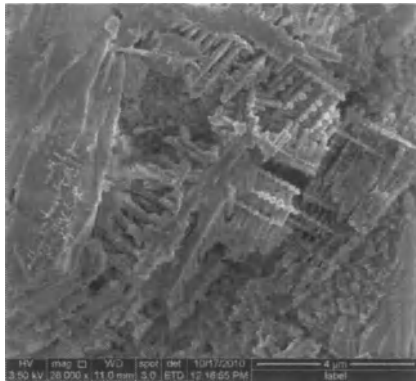
Figure 14. SEM photomicrograph of amorphous and crystalline polymerized phases (75% tuff).
