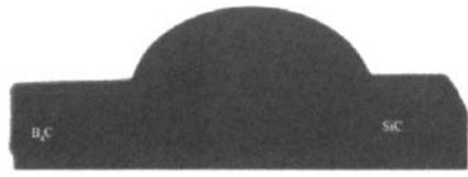
Experiment 5 - photo 04 - B_2O_3 on ( B_4C / SiC ) - 553^\circ C
