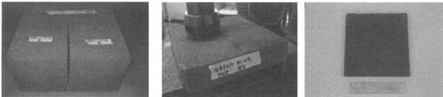
Figure 1. Machining of graphitic foam cores.
