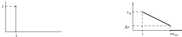
**Fig. 3.** Dirac impulse and a system response
