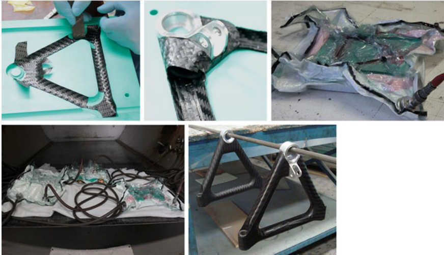
Fig. 11 Production sequence of upper wishbone
