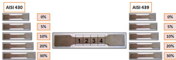
Fig. 1 Scheme of section of the test specimen for obtaining samples to be nitrided
