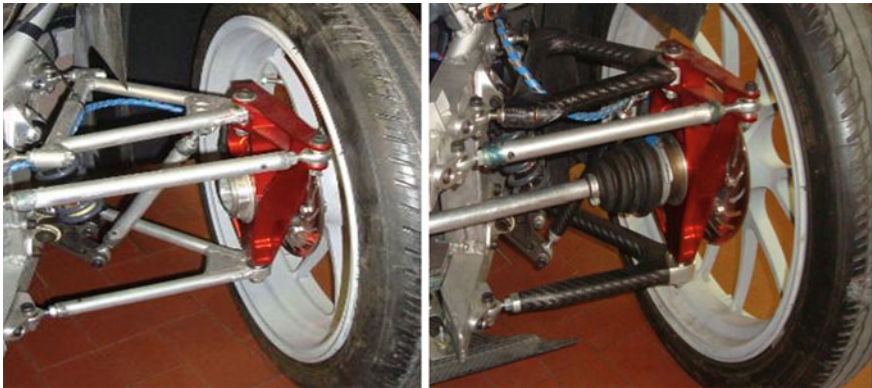
Fig. 12 The solution in aluminum on XAM 1.0 ( on the left ) and solution in carbon fiber on XAM 2.0 ( on the right )
