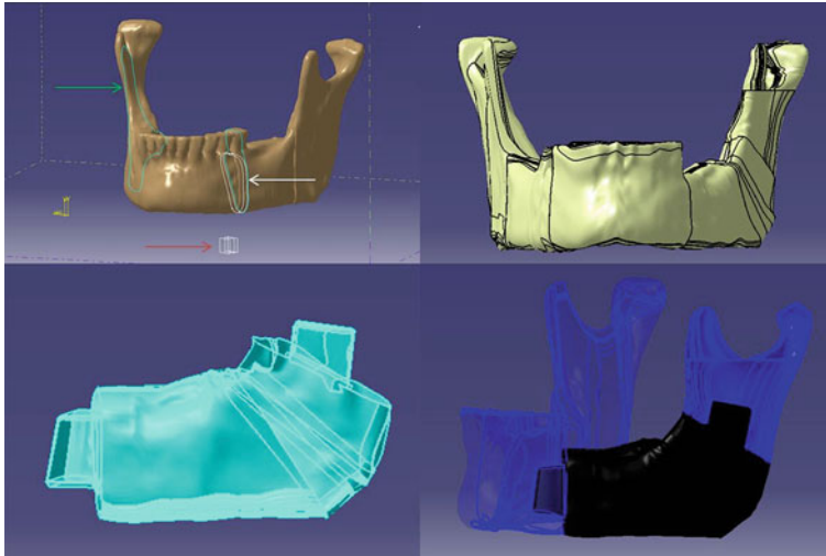
Fig. 9 3D model exported from Scan IP® displaying auxiliary paths ( green arrow ), planes ( red arrow ) and cross sectional sketches ( white arrow ) ( top left ); surface model created through a series of sketches ( top left ); final design of prosthetic device ( bottom left ) and prosthesis final design including adjacent bone regions from the mandible of patient B ( bottom right )
