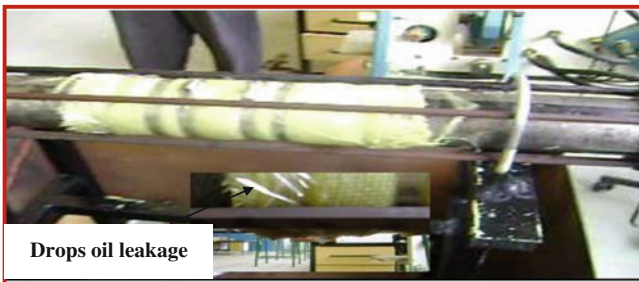
Fig. 10 Photograph of circumferential delimitation failure for rectangular defect (7 × 14) mm
