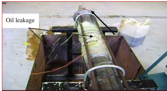
Fig. 9 Photograph of failure at centre of the rectangular defect (9 × 18) mm
