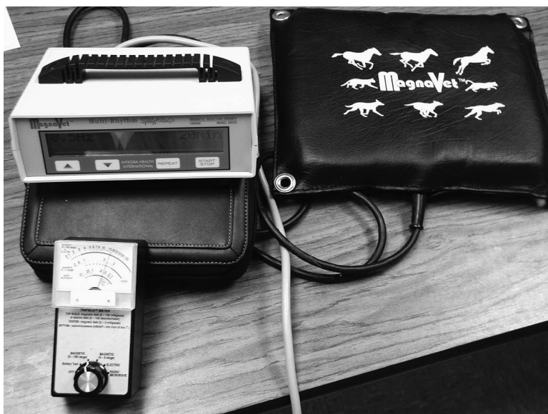
FIG. 16-11. A pulsed electromagnetic field generator designed for animals.
