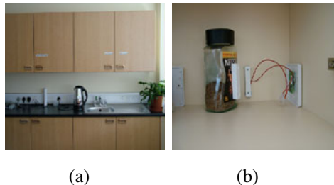
Fig. 3. The smart kitchen laboratory in the University of Ulster at Jordanstown: (a) an overall kitchen view; (b) a coffee jar attached with a contact sensor
