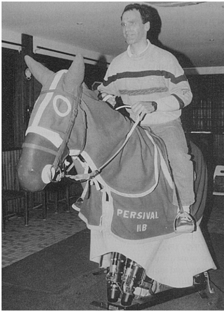
Figure 1.7 Persival, the Ecole Nationale d'Equitation's mechanical horse simulator.
