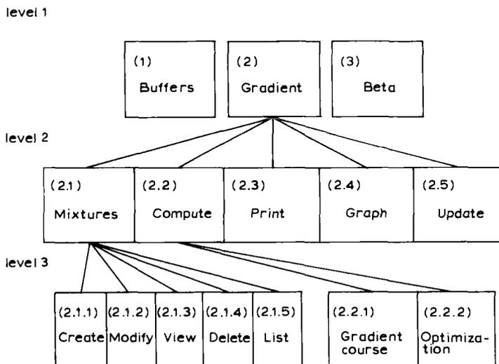
Fig. 2.14. An overview of the structure of the automatic program for pH gradient,  $\beta$  and I simulation in IPGs. Notice the tree-like organization inherent to the Pascal language (from Celentano et al., 1987; with permission of Elsevier).
