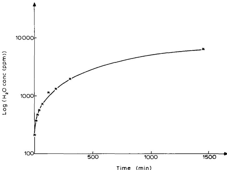
Fig. 1.22. Absorption of water in *n*-propanol from air, at 40% relative humidity at room temperature. Water content assessed by the Karl-Fischer method (from Gäveby et al., 1988; by permission of Elsevier).
