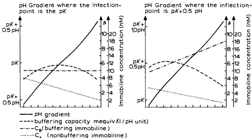
Fig. 2.2. pH gradients with midpoint ( $pH_m$ ) centred or removed from the buffer  $pK$ . Left: the simple case in which  $pH_m = pK$ ; right: extreme case in which  $pH_m = (pK + 0.5 \text{ pH unit})$ . Solid lines: pH gradients; broken curves:  $\beta$  power courses; broken and dotted lines: concentration courses of buffering Immobilines; dotted lines: concentration profiles of titrant Immobilines (courtesy of LKB Produkter AB).
