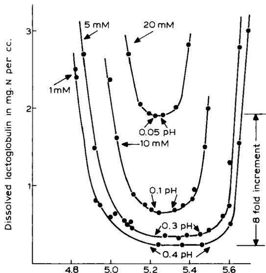
Fig. 5.4. Solubility of  $\beta$ -lactoglobulin in the pH range 4.8–5.6 as a function of the ionic strength of the environment, from 1 mM to 20 mM NaCl. The amount of protein dissolved has been determined as Kjeldhall nitrogen. The pH values on the parabolas give the span of the solubility minimum, centred on a theoretical pI of 5.3 (modified from Grönwall, 1942).
