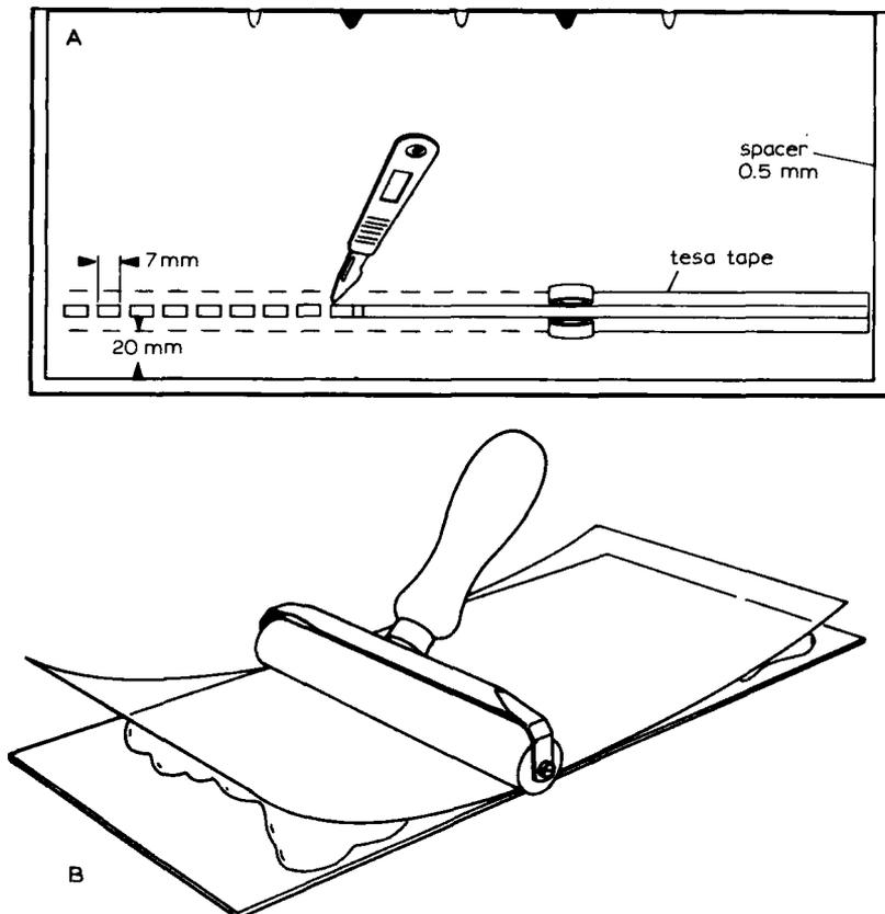
Fig. 3.2. Preparation of the gel cassette. (A) preparation of the slot former: onto the cover plate (bearing the rubber gasket U-frame) is glued a strip of tesa tape out of which rectangular tabs are cut with a scalpel. (B) application of the Gel Bond PAG film to the supporting glass plate. (C) assembling the gel cassette (courtesy of LKB Produkter AB).
