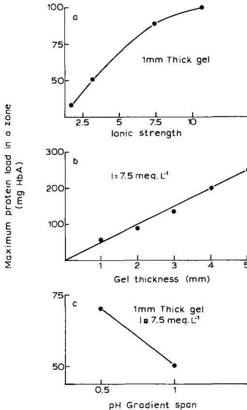
Fig. 5.3. Loading capacity of IPGs. The maximum load in a single protein zone is plotted: (a) as a function of gel thickness at constant ionic strength in a 1 pH unit interval; (b) as a function of gel thickness at constant  $I$  in a 1 pH unit interval; (c) as a function of pH gradient width at constant  $I$  and constant gel thickness (from Gelfi and Righetti, 1983; with permission from Elsevier).
