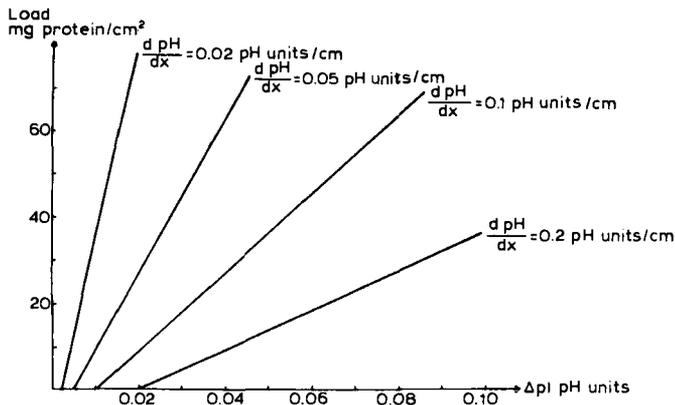
Fig. 5.2. Acceptable protein load (mg/cm<sup>2</sup>) as a function of  $\Delta pI$  for different pH slopes plotted for a mean concentration of 45 mg/ml in the major protein zone. This is a graphical representation of Eqn. (1) (from Ek et al., 1983; by permission from Elsevier).
