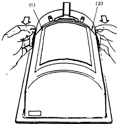
Fig. 3.17. Drawing of the commercial gel slicer from Pharmacia-LKB. The IPG gel, pasted to the Gel Bond PAG foil, is fastened to the curved shield (1). With a quick hand movement, the steel wire (2) is slid at the interface between the IPG matrix and the supporting plastic foil.
