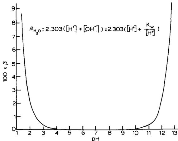
Fig. 2.17. Buffering power ( $\beta$ ) of water along the pH axis. For calculations, we have taken as  $pK$  of the base  $H^+$  the value of  $-1.74$  and as  $pK$  of the conjugated acid  $OH^-$  the value of  $15.74$  (the molarity of water being  $55.56$ ).  $K_w$  is the ionic product of water. It is seen that water does not have any appreciable buffering power in the pH 4–10 interval. Calculations and simulations according to the new computer program of Celentano et al. (1988).
