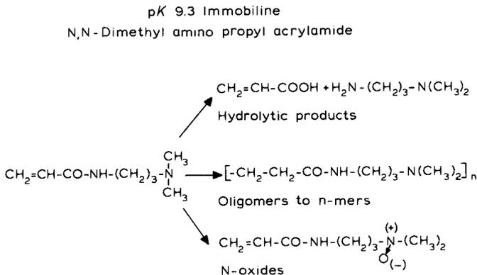
Fig. 1.15. Demonstration of the three degradation pathways of alkaline Immobilines, exemplified by the example of the pK 9.3 species. Note that the first two degradation processes are in common with the acidic Immobilines, while the oxidation phenomenon only occurs with the alkaline compounds.
