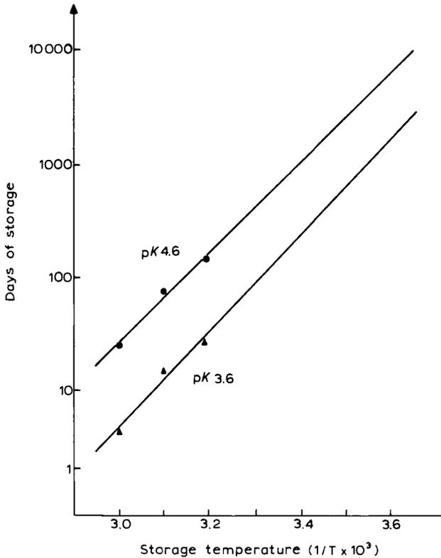
Fig. 1.21. Arrhenius plot showing how many days Immobilines pK 3.6 (▲▲▲) and pK 4.6 (●●●) can be stored at different temperatures as 0.2 M solutions in water (containing 5 ppm inhibitor) before the acrylic acid concentration reaches 1 mole-% of the Immobililine level. From extrapolated data, it appears that the pK 3.6 can be stored 1200 days and the pK 4.6 species 4800 days at +8°C (from Gäveby et al., 1988; with permission of Elsevier).
