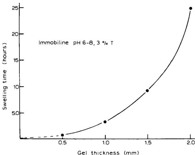
Fig. 3.4. Swelling kinetics of Immobiline gels. The equilibrium swelling times of gels of various thicknesses have been plotted against gel thickness for 3%  $T$ , pH 6–8 Immobiline gels. Notice how the exponential becomes very steep above 1 mm thickness (from Gelfi and Righetti, 1984; with permission of Verlag Chemie).
