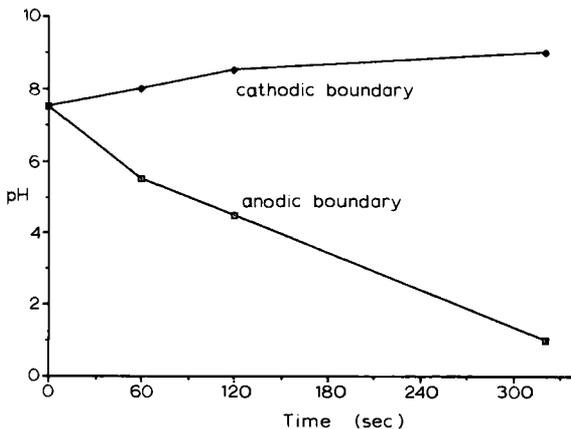
Fig. 3.25. Assessment of pH of salt ion boundaries in the sample zone. Pockets cast in the gel middle (pH 7.5) were filled with 20  $\mu$ l of 100 mM NaCl. The cathodic and anodic edges were covered with strips of alkaline and acidic pH indicators, respectively. The pH in the two boundaries was assessed by visual inspection of color changes at the given time intervals at constant 2000 V (from Righetti et al., 1988e; with permission of Verlag Chemie).
