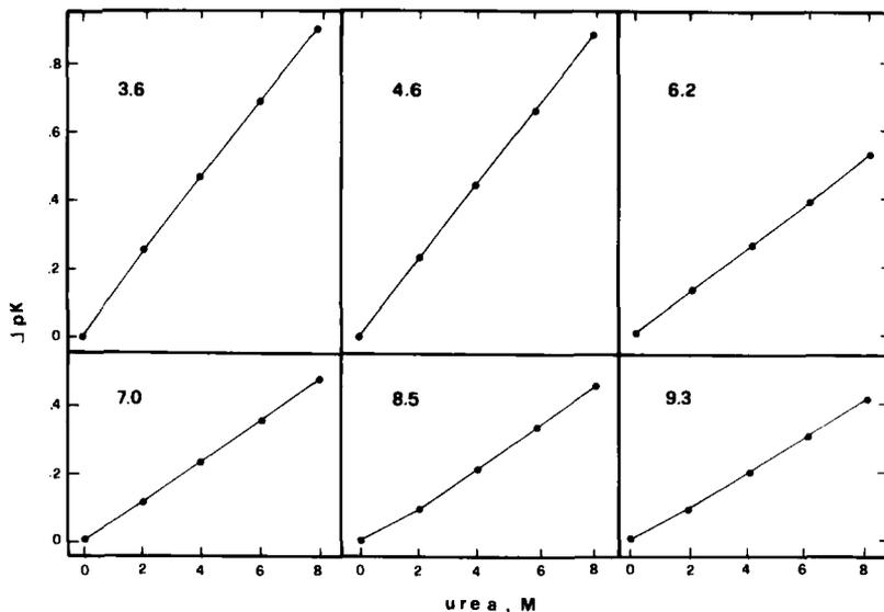
Fig. 1.7. Dependence of Immobiline pKs on urea concentration. A 20 mM solution of each Immobiline was titrated to its pK (with Immobiline of pK 3.6 or 9.3 as counter-ion). Aliquots of this stock solution were diluted to a 10 mM concentration in the presence of various amounts of urea. pH readings were made at 20°C.  $\Delta pK$  refers to  $pK_{\text{urea}} - pK_{\text{water}}$  (from Gianazza et al., 1983c; with permission of Verlag Chemie).
