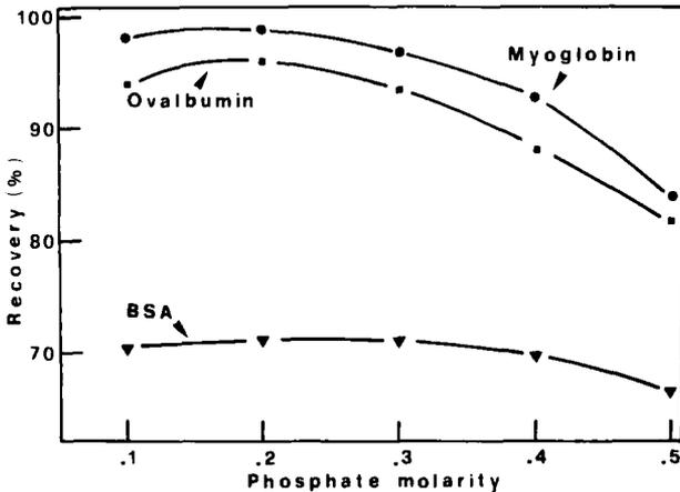
Fig. 5.14. Recovery of protein fractions from HA-Ultrogel as a function of phosphate eluant molarity. Myoglobin (circles), ovalbumin (squares) and BSA (triangles) were separately adsorbed onto hydroxyapatite, equilibrated in 100 mM Tris-Gly buffer, pH 9.1, and eluted with increasing molarities (from 0.1 to 0.5) of pH 6.8 phosphate buffer (from Ek et al., 1983; with permission from Elsevier).
