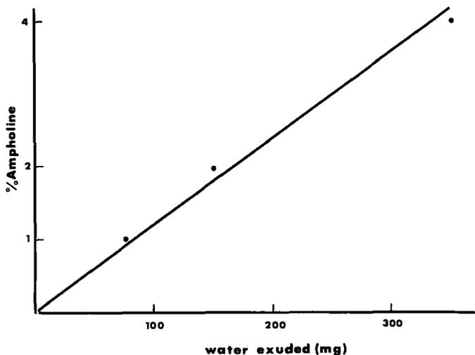
Fig. 3.23. Water exudation as a function of level of carrier ampholyte in the Immobiline gel. A 5% T, 4% C IPG gel, in the pH 4–8 range, was polymerized, washed, dried, divided into three identical strips (8 cm wide, 11 cm long, 1 mm thick) and re-swollen in 1%, 2% or 4% Ampholine in the pH 4–8 range. After focusing for 6 h at 2000 V (at equilibrium), the total water exuded by each gel was carefully blotted and weighed (from Astrua-Testori and Righetti, 1987; with permission of Elsevier).
