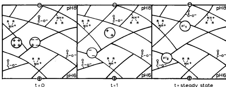
Fig. 1.3. The third IEF generation: immobilized pH gradients. Note that at all stages of electrophoresis ( $t=0$  to  $t = \text{steady-state}$ , the pH gradient is already fully established and immobile in the electric field. Thus, only the proteins keep migrating under the applied voltage till reaching a steady-state (modified from an erroneous drawing in the LKB catalog, 1987).
