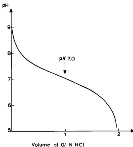
Fig. 2.1. Titration of  $pK$  7.0 Immobiline with 0.1 M hydrochloric acid. If the buffering Immobiline concentration is kept constant, the titration curve produces a linear gradient within  $pK + 0.5$  pH unit and  $pK - 0.5$  pH unit (i.e., 1 pH unit interval having the  $pK$  value as inflection point) (by courtesy of LKB Produkter AB).
