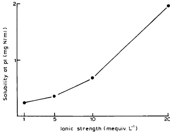
Fig. 5.5. Plot of solubility at pI vs. ionic strength of the milieu for  $\beta$ -lactoglobulin. Data from Fig. 5.4. The solubility increases by a factor of 8 for a 20-fold increase in ionic strength (Gelfi and Righetti, unpublished).
