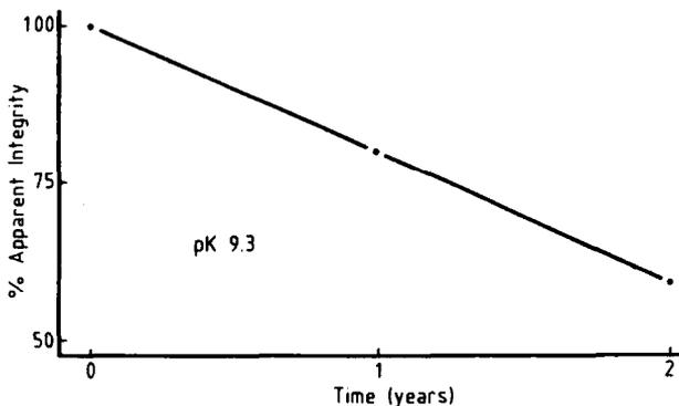
Fig. 1.11. Decay kinetics of the pK 9.3 Immobiline. A 0.2 M water solution of this buffer was kept frozen at  $-20^{\circ}\text{C}$  over a 2-year period and analyzed at 1-year intervals. For calculating the percentage of hydrolysis, the pI shifts of a train of myosin light chains were used to obtain the modified pH intervals with the aid of the adapted H-H Eqn. 3 (from Astrua-Testori et al., 1986; with permission of Verlag Chemie).
