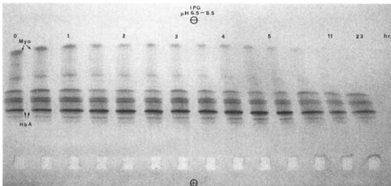
Fig. 5.25. Purification of Hb A from myoglobin in a segmented IPG gel. An experiment similar to that of Fig. 5.24 was run. Purified Hb A (50 mg) was mixed with 20 mg of sperm whale myoglobin (Myo) and recycled for 23 h at 1000 V, 3 mA, 3 W. 30  $\mu$ l aliquots were analyzed at the given time intervals in an analytical IPG gel in the pH 6.5–8.5 range (from Faupel et al., 1987; with permission from Elsevier).
