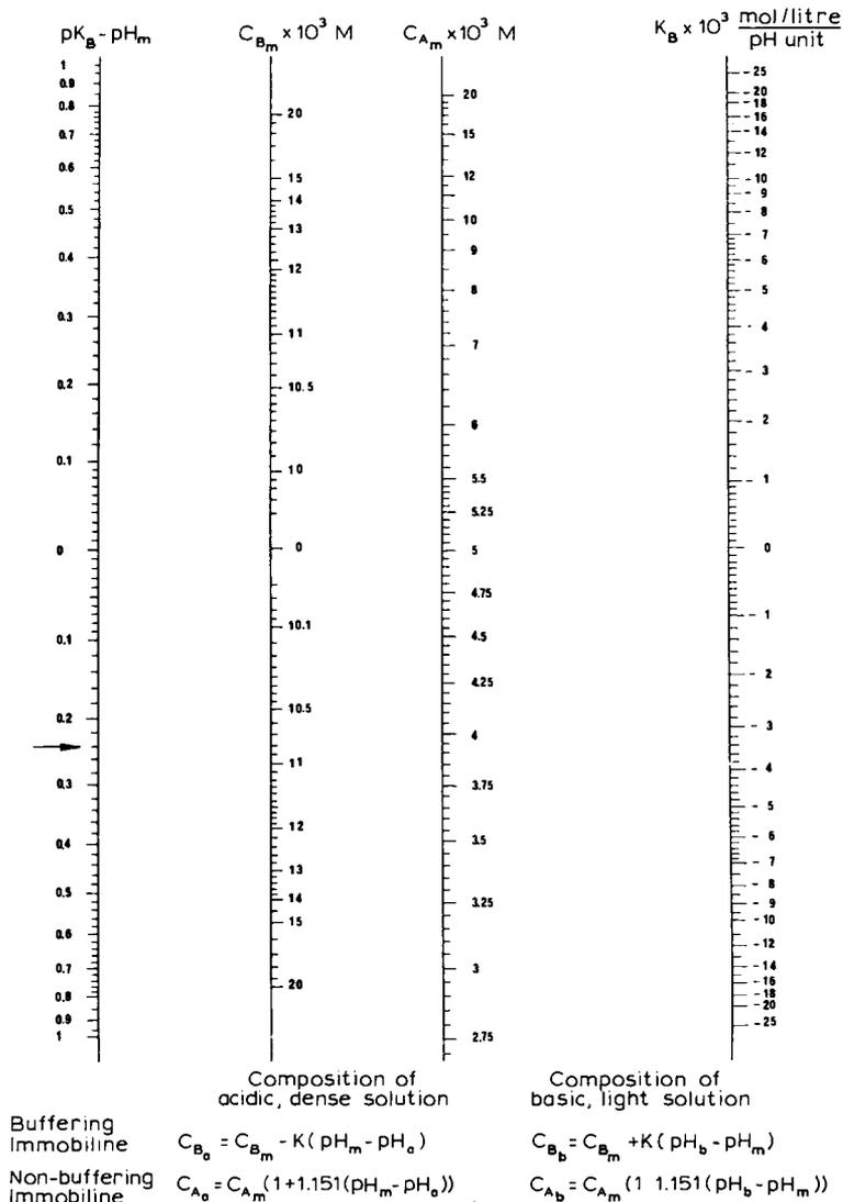
Fig. 2.4. Nomogram No. 2, to be used to calculate the amounts of buffering and titrant Immobilines in the dense and light solutions in the case in which the buffering species is a base. For its use, see the example in the text and follow the general instructions in LKB Application Note No. 321 (1982) (by courtesy of LKB Produkter AB).
