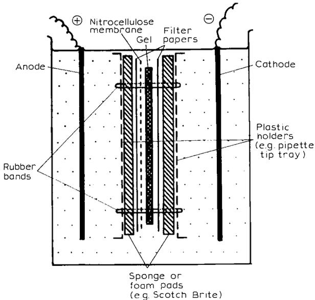
Fig. 3.18. 'Western blotting', i.e. electrophoretic transfer of macromolecules from a gel slab to an immobilizing membrane. Diagram showing a typical transfer assembly (from Andrews, 1986; by permission of Clarendon Press).
