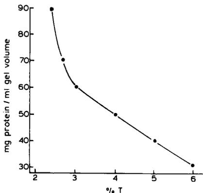
Fig. 5.9. Relation between loading capacity (in terms of mg protein/ml gel volume) and %  $T$  ( $T$  = grams of acrylamide and cross-linker per 100 ml gel volume) value of the gel matrix. Notice that, while in the range 3% to 6%  $T$  the protein load decreases linearly, in softer gels ( $C$  3%  $T$ ) it increases exponentially (from Righetti and Gelfi, 1984; with permission from Elsevier).
