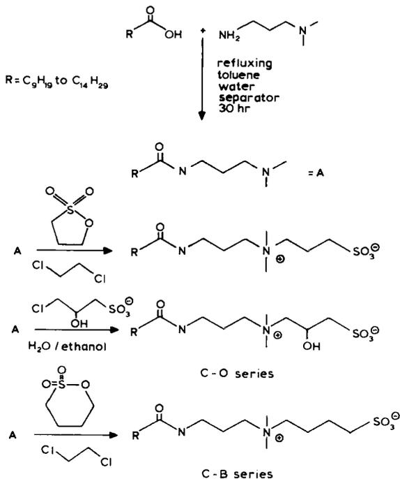
Fig. 4.1. Synthesis of new surfactants. Upper: fatty acids (R-OOH) are reacted with *N,N*-dimethyl 1,3-propanediamine to form an amido amine (A). Compound A is reacted: (I) with propan sultone to produce the C-series; (II) with Na 3-chloro 2-hydroxy propanesulfonate to generate the C-O series and (III) with butane sultone to give the C-B-series (from Rabilloud et al., 1988b; by permission from VCH).
