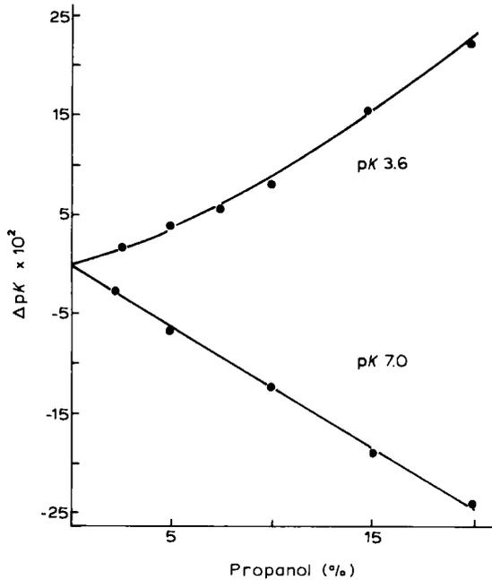
Fig. 1.24.  $pK$  shifts of one acidic ( $pK$  3.6) and one alkaline ( $pK$  7.0) Immobiline as a function of % *n*-propanol in water. The  $pK$  shifts have been determined by measuring the pH of solutions titrated to the  $pK$  value (2:1 molar ratio buffer:titrant) in presence of different amounts of *n*-propanol in water at 25°C. The concentrations used were 10 mM for the buffering group and 5 mM for the titrant (from Gåveby et al., 1988; with permission of Elsevier).
