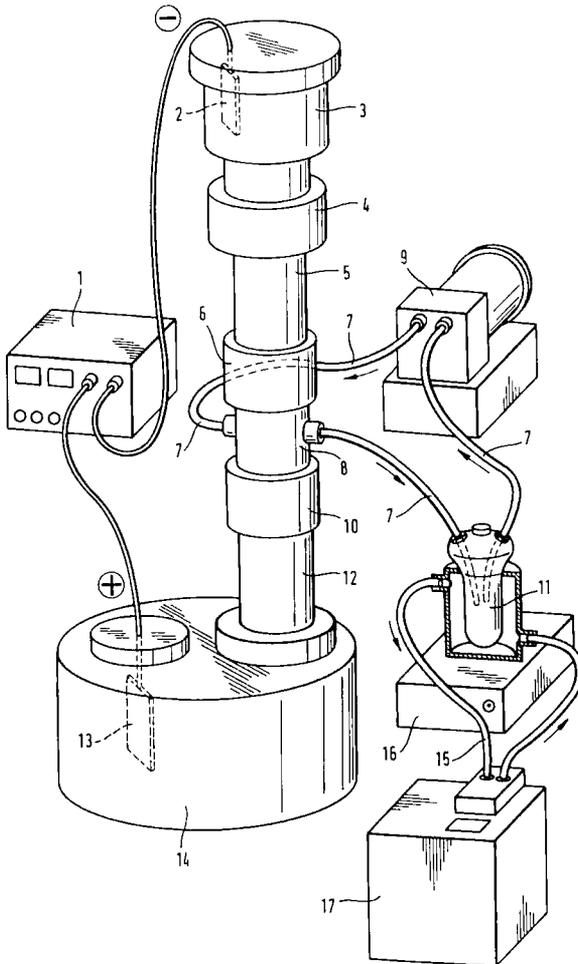
Fig. 5.22. Experimental assembly of a preparative IPG run in a segmented gel apparatus. 1: power supply; 15: tubing for the coolant flow to the sample reservoir (11); 16: motor for magnetic stirring; 17: thermostat. All other numbers as in Fig. 5.21 (modified from Faupel et al., 1987).
