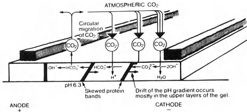
Fig. 2.16. Diagram illustrating the principle of interference by atmospheric carbon dioxide at high pH. Hypothetical cross-section of a gel. Note that, at pH 10 and above the  $\text{CO}_3^{2-}$  ion predominates, whereas between pH 6.3 and 10.3 the  $\text{HCO}_3^-$  is the most abundant species. Below pH 6, the adsorbed  $\text{CO}_2$  is released back in the atmosphere as gaseous carbon dioxide (from Burdett, 1982; by courtesy of Pharmacia Fine Chemicals).
