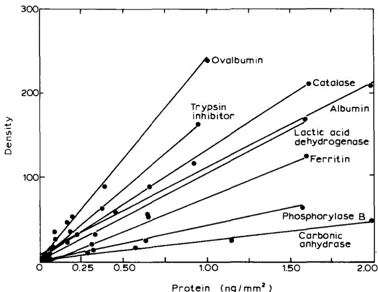
Fig. 4.16. Silver stain density versus protein concentration for purified proteins (Pharmacia markers) electrophoresed in 10% *T* polyacrylamide gels (0.88 mm thick) at 20 mA/gel. The gel images were developed for 9 min in sodium carbonate-formaldehyde solution. Band areas and densities were measured by computerized densitometry (from Merril and Goldman, 1984).
