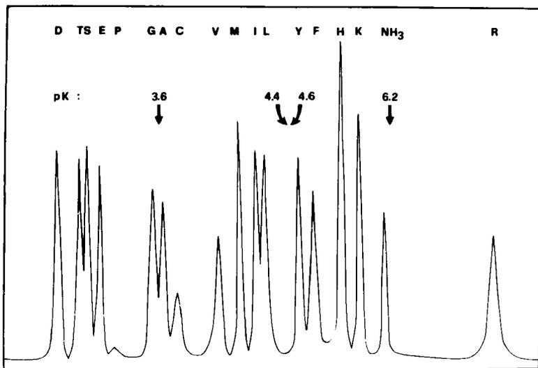
Fig. 1.9. Interference from Immobilines in amino acid analysis. A sample of each Immobiline was hydrolyzed and run on an ion-exchange automatic chromatograph for amino acid analysis. The elution profiles of their split products are shown by arrows on a typical chromatogram of natural amino acids, which are identified by their one-letter symbols in the top row (from Gianazza et al., 1983b; with permission of Elsevier).
