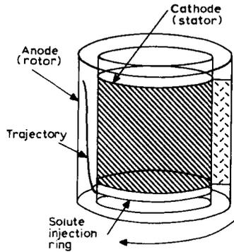
Fig. 5.33. Scheme of the Biostream separator. Protein separation occurs in an annulus between a static cathode and a rotating anode. Carrier fluid flows axially upwards through the annulus and feed is injected through a ring-shaped opening just below the electrodes. The liquid is collected into 50 fractions at the top.
