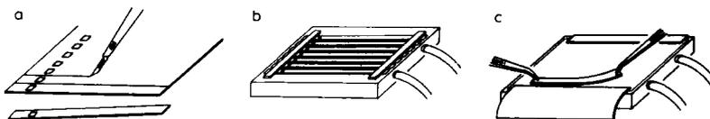
Fig. 4.7. IEF in individual IPG gel strips on Gel Bond PAG film. Strips were cut from the washed and dried IPG gel or ready-made IPG dry plates, rehydrated and placed on the cooling block of the electrophoresis chamber. Sample solution is pipetted into a silicone rubber frame (from Görg et al., 1988b; with permission from VCH).
