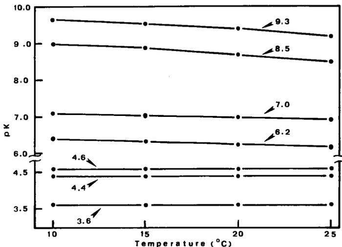
Fig. 1.6. Temperature coefficients ( $dpK/dT$ ) for the seven Immobiline chemicals in the temperature range 10–25°C (from Righetti et al., 1983a; with permission of Elsevier).
