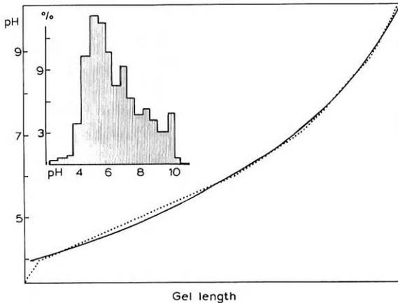
Fig. 2.10. Non-linear pH 4–10 gradient. Dotted line: ideal; solid line: actual (lower formulation, including acidic titrant from Table 2.6) pH courses. The shape for the ideal profile was computed from data on the statistical distribution of protein pIs (Gianazza and Righetti, 1980). The relevant histogram is redrawn in the figure inset (from Gianazza et al., 1985b; with permission from Verlag Chemie).
