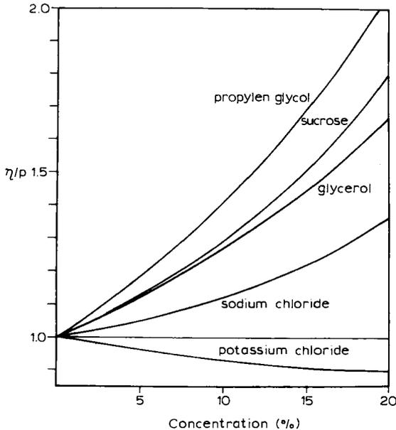
Fig. 3.8. Plot of  $\eta/\rho$  versus concentration for some common chemicals.  $\eta$ , relative viscosity;  $\rho$ , relative density. The thin horizontal line is an ideal line with zero slope (from Dossi et al., 1983; with permission of Elsevier).
