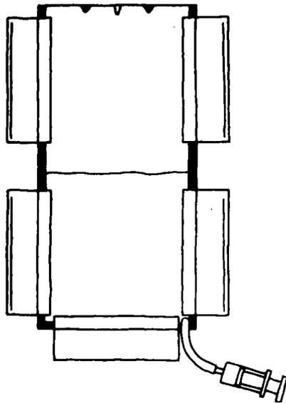
Fig. 3.7. Re-swelling cassette for dry IPG gels. The dried IPG gel (on its plastic backing) is inserted in the cassette, which is then gently filled with any desired re-swelling solution via a bottom hole (by courtesy of LKB Produkter AB).
