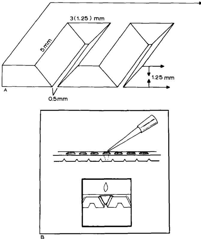
Fig. 3.14. Top (A) and bottom (B) of the sample applicator strip commercially available from Pharmacia-LKB. The applicator contains 53 slots (each  $5 \times 1 \times 1$  mm) separated by slits (parallel to the slots) 1 mm wide. A: from Pflug (1988b) with permission of VCH; B: by courtesy of Pharmacia-LKB.
