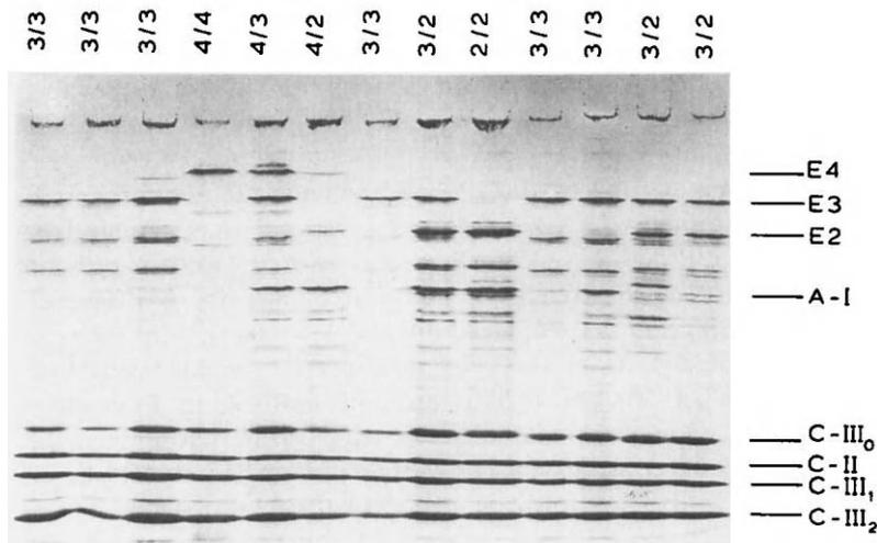
Fig. 6.14. IEF of apolipoproteins from VLDL in a CA-IPG system. For each lane, apo E phenotypes are indicated. Staining with Coomassie Brilliant Blue R-250. The gel (pH 4-7 range) was re-swollen in 8 M urea, 30% glycerol, 2 mM Tris and 1% Servalyt pH 4-7. Cathodic sample application (at the top in the figure). Focusing conditions: overnight at 5000 V, 3 mA, 3 W with a Macrodrive power supply at 15°C (from Baumstark et al., 1988; with permission from VCH).
