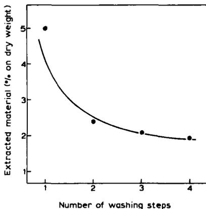
Fig. 3.12. Efficacy of repeated washing steps on the reduction of extractable material from IPGs. IPGs in the pH range 5.4–6.4 were washed in distilled water (500 ml per 20 ml of gel) 1–4 times, 30 min each. The gel was then extracted with 80% acetic acid and the supernatant dried to constant weight on KOH (from Gianazza et al., 1983b; with permission of Elsevier).
