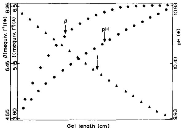
Fig. 2.21. Computer simulation of an Immobilized pH 10–11 gradient. Buffering Immobililine:  $pK$  10.3; titrant Immobililine:  $pK$  3.6 (see recipe in Table 2.9). The values of pH, buffering power ( $\beta$ ) and ionic strength ( $I$ ) are calculated at 0.05 pH increments according to Celentano et al. (1987) (from Gelfi et al., 1987b; with permission of Elsevier).
