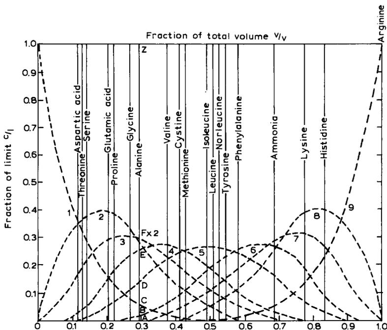
Fig. 2.6. Composition of the eluate from a nine-chambered gradient in terms of the contribution of each buffer in a single chamber (numbered 1-9). The vertical lines represent the elution position of each amino acid from the Autoanalyzer when using a Varigrad for mixing the eluent buffers (modified from Peterson and Sober, 1959).
