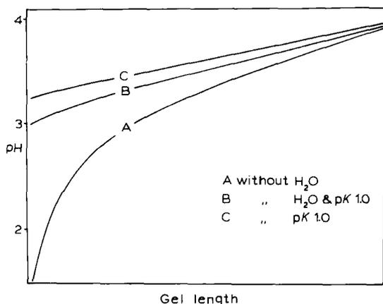
Fig. 2.19. Simulated pH gradients in the absence of some components from the recipe for the pH 3–4 gradient in Table 2.10. A: pH gradient in the absence of the ‘Immobiline’ water (1 M); B: pH gradient obtained by the simultaneous subtraction of water and Immobiline pK 1.0; C: pH gradient without the Immobiline pK 1.0 in the formulation (from Righetti et al., 1986c; by permission of Elsevier).
