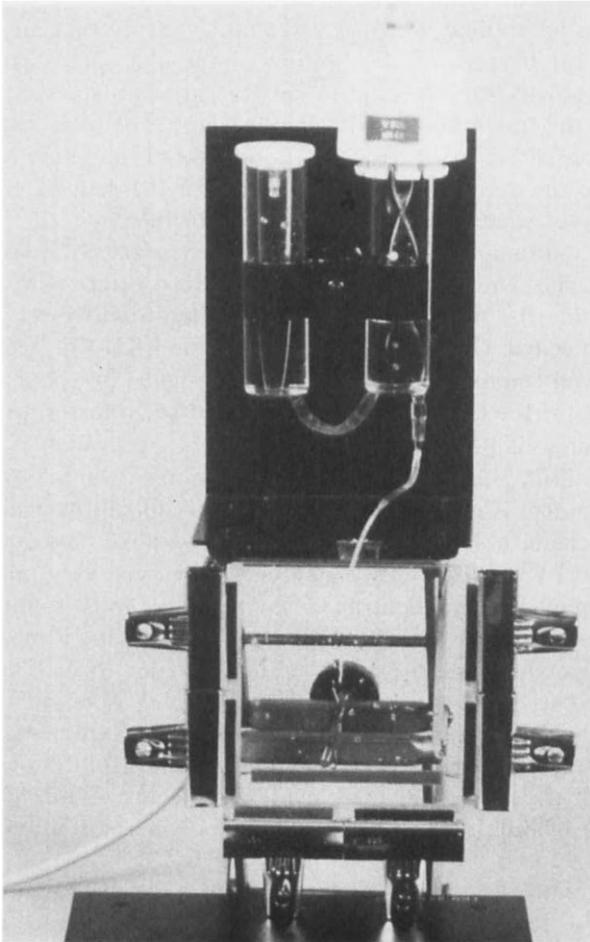
Fig. 5.11. Equipment needed for casting a 5-mm thick IPG gel slab. The glass tray is 1/2 the size of the cooling block of the electrophoresis chamber, and contains a U-gasket of silicone, 5 mm thick. A sample application trench is created by building up layers of embossing tape (10–12 layers of Dymo tape) on the glass. For pouring the gradient, the LKB 8121 Gradient Mixer and 8123 Stirrer Motor from the old sucrose density gradient column for IEF is used (60 ml total volume/chamber).
