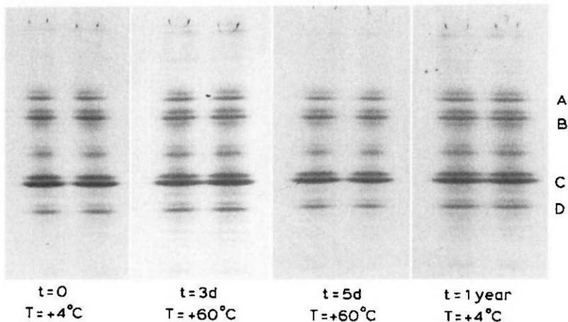
Fig. 1.20. IEF of ovalbumin in a pH 4.28–4.90 IPG range. The gel was made with Immobiline pK 4.6 as buffer and Immobiline pK 8.5 as titrant. The latter was dissolved in *n*-propanol (containing < 500 ppm H<sub>2</sub>O) and incubated 3 or 5 days at 60°C or 1 year at 4°C. Note the identical banding patterns under all storage conditions (from Gåveby et al., 1988; with permission of Elsevier).
