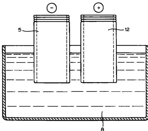
Fig. 5.32. Sketch of a 'tower' IPG apparatus. The sample is kept in a large, stirred and cooled reservoir (8), into which two cylinders (5 and 12) are lowered, containing either IPG gel intervals or IPG pH plateaus (membranes) for removal of non-iso-electric impurities. The catholyte and anolyte are poured on top of the IPG gel layers in cylinders 5 and 12; the Pt electrodes are not shown (Righetti and Faupel, unpublished).
