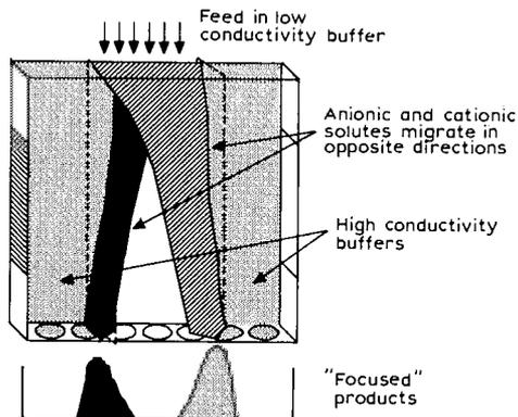
Fig. 5.35. Scheme of the Wagner's apparatus for field step focusing. The sample is introduced in a thin electrophoresis cell (continuous flow, curtain type) as a broad, low conductivity curtain. Sample components are forced to 'focus' against two lateral, high conductivity buffers. The pH of the central curtain is adjusted so that it is intermediate between the pIs of two 'key' components whose purification is sought.
