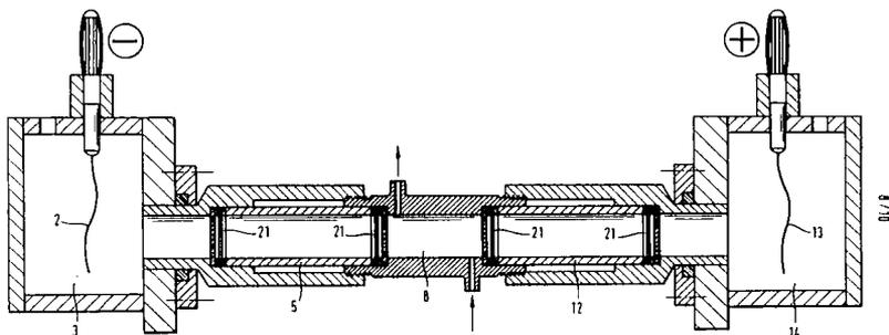
Fig. 5.26. Sketch of the horizontal, segmented IPG apparatus. 2 and 13: platinum wires; 3 and 14: electrolyte reservoirs; 5 and 12: plastic cylinders for holding the IPG gel segments (polymerized in glass tubes and subsequently inserted in these sleeves); 8: sample flow chamber; 21: membranes bound to the extremities of the IPG gel segments (modified from Righetti et al., 1987f).
