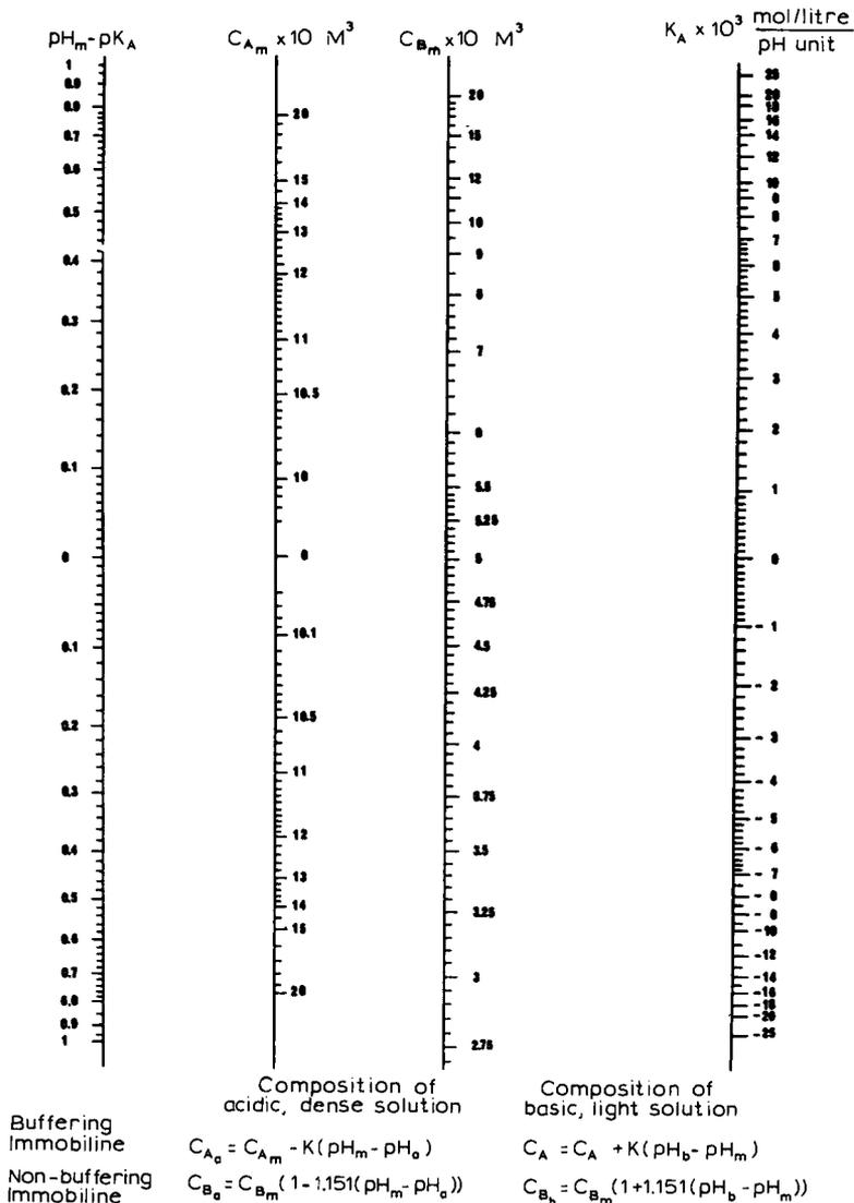
Fig. 2.3. Nomogram No. 1, to be used to calculate the amounts of buffering and titrating Immobilines in the dense and light solutions in the case in which the buffering species is an acid. For its use, see the practical example in the text (from LKB Application Note No. 321, 1982; by courtesy of LKB Produkter AB).
