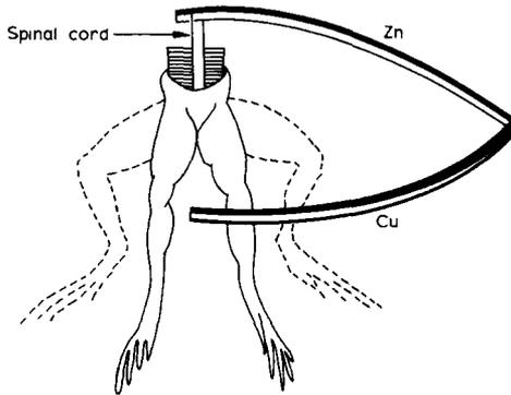
Fig. 0.2. The classical ‘frog-leg’ experiment of Luigi Galvani. When an arc was made between the spinal nerve and a pair of skinned frog legs, the legs would contract (dotted profile) each time the circuit (made by two pieces of Cu and Zn, joined in the middle) was closed. Galvani’s interpretation: ‘animal electricity’. Volta’s interpretation: potential difference (voltage, to be sure) generated at the contact between two unlike metals.
