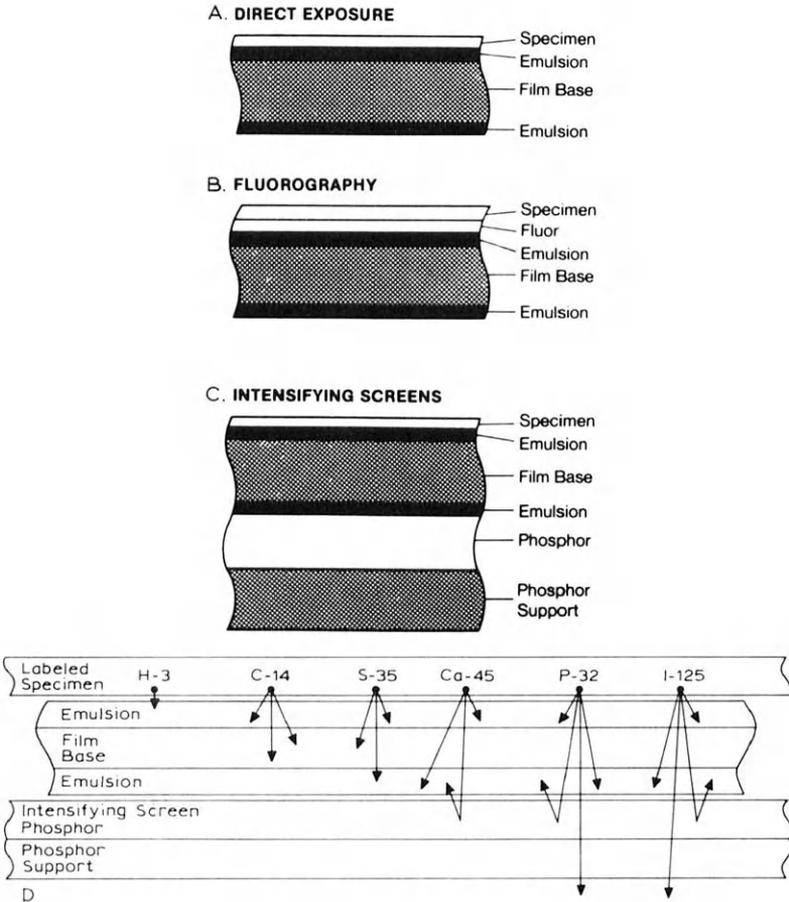
Fig. 3.28. The three classical methods of autoradiography. (A): by direct exposure; (B): by fluorography and (C): with the use of intensifying screens. (D) illustrates the penetration of different radiations into X-ray film. Note that the intensifying screen phosphor method can only be used with high-energy emitters (e.g., gamma radiations) as they can penetrate through the film and excite the phosphor underneath (by courtesy of Eastman Kodak Company).
