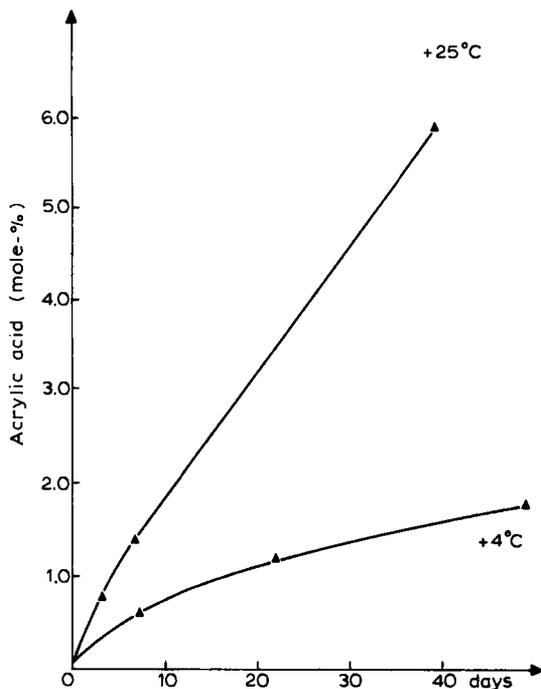
Fig. 1.19. Mole-% of acrylic acid formed in Immobiline  $pK$  8.5 as 0.2 M solution in water at  $+4^{\circ}\text{C}$  and at room temperature as a function of time. The acrylic acid concentration was determined by isotachopheresis (from Gäveby et al., 1988; by permission of Elsevier).
