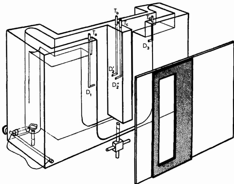
Fig. 1.1. The first IEF generation: pH gradients generated by diffusion followed by electrophoretic protein transport. Perspective view of the Kolin electrophoretic fractionation cell.  $T_a$ ,  $T_b$ ,  $T_c$  and  $T_d$ : hypodermic syringe tubings.  $D_1$ ,  $D_2'$ ,  $D_2''$  and  $D_3$ : corresponding horizontal ducts (by courtesy of Dr. A. Kolin).
