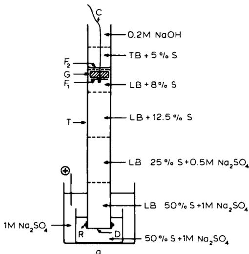
Fig. 5.18. Elution of protein bands by a combination of displacement electrophoresis and electrophoresis in a conductivity gradient. TB: terminating buffer; LB: leading electrolyte; S: sucrose solution; G: Immobiline gel slice; E<sub>1</sub> and E<sub>2</sub>: electrode vessels; D: dialysis membrane; R: rubber band; F<sub>1</sub> and F<sub>2</sub>: filter paper; C: cotton thread (adapted from Hjertén et al., 1983; with permission from Elsevier).
