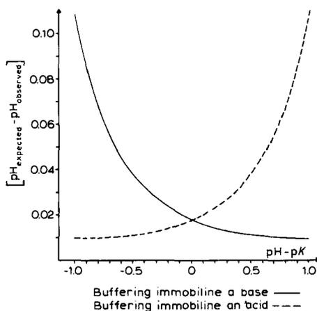
Fig. 2.15. Effect of a 2% error in dispensing the Immobilines on the pH of the solution, in relation to the  $pK$  of the buffering base and the buffering acid. Note how, in both cases, a very low experimental error is produced in the proximity of the  $pK$  values ( $pH - pK = 0$ ) (from LKB Application Note No. 321; by courtesy of LKB Produkter AB).
