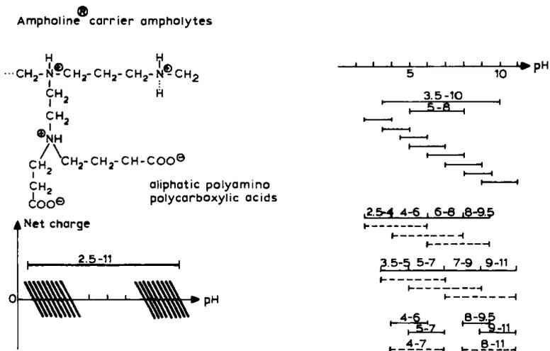
Fig. 1.5. Composition of Ampholine. On the upper left side a representative chemical formula is shown (aliphatic oligo amino oligo carboxylic acids). On the lower left side, portions of hypothetical titration curves of Ampholines are depicted. Right: different pH cuts for wide and narrow range carrier ampholytes (courtesy of LKB Produkter AB).
