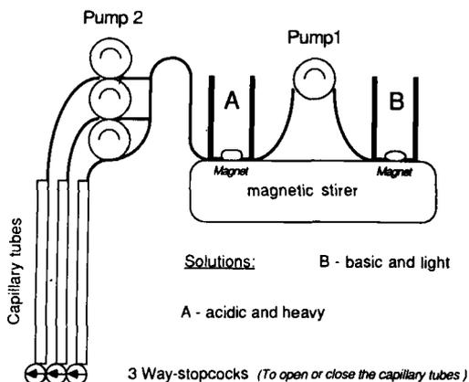
Fig. 4.11. Preparation of cylindrical IPG gels. The solution from reservoir B is transferred by pump 1 to the mixing chamber (A). A multichannel pump (Ismatec, Zurich) conveys the gradient solution simultaneously to the top of 20 glass tubes (200 × 1.5 mm i.d.) standing vertically (from Hochstrasser et al., 1986b).
