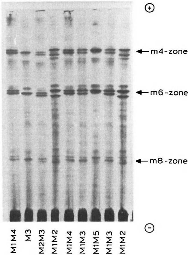
Fig. 6.13. Demonstration of PI-M subtypes as analyzed by IEF in IPGs, in a pH 4.3–4.8 range, over a 17 cm electrode distance, giving a  $\Delta\text{pH} = 0.025/\text{cm}$ . Cathodic sample application in  $6 \times 6 \times 0.25$  mm slots. Coomassie Blue staining (from Görg et al., 1985a; with permission from the Amer. Soc. Hum. Genet.).
