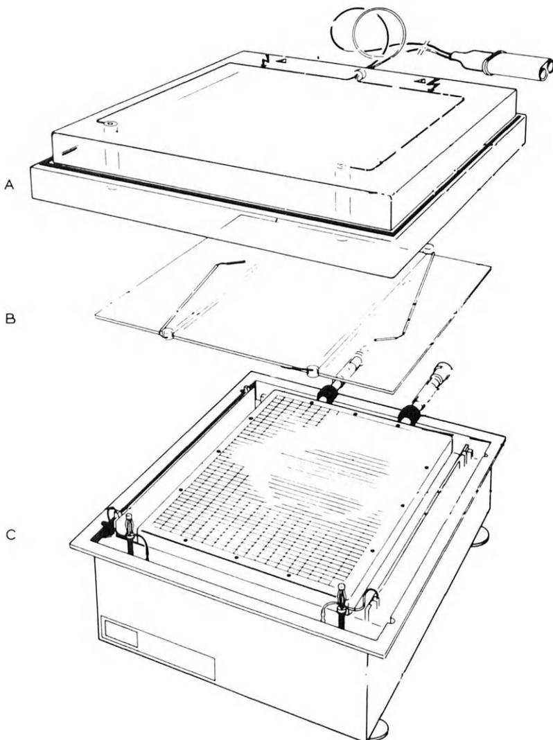
Fig. 3.1. Drawing of the LKB Multiphor II chamber. (A) cover lid; (B) cover plate with movable platinum electrodes; (C) base-chamber with ceramic cooling block for supporting the gel slab (courtesy of LKB Produkter AB).
