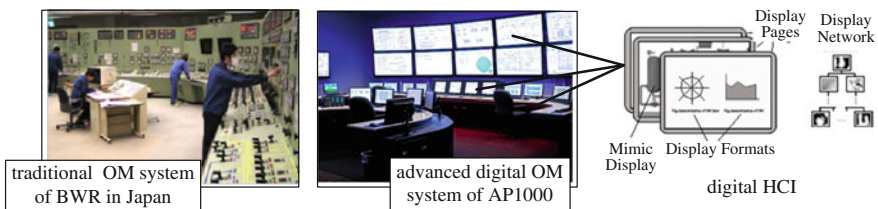
Fig. 46.1 Case of the traditional OM system and the advanced digital OM system of AP1000
