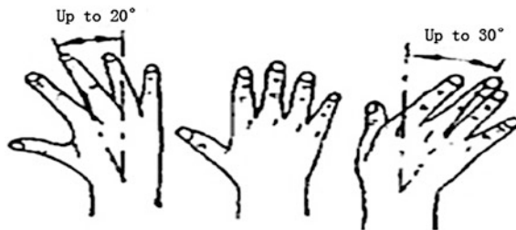
Fig. 82.4 Fingers conversion angle. Reprinted from Ergonomics . [255], Copyright 2008, with permission from Beijing Institute of Technology Press
